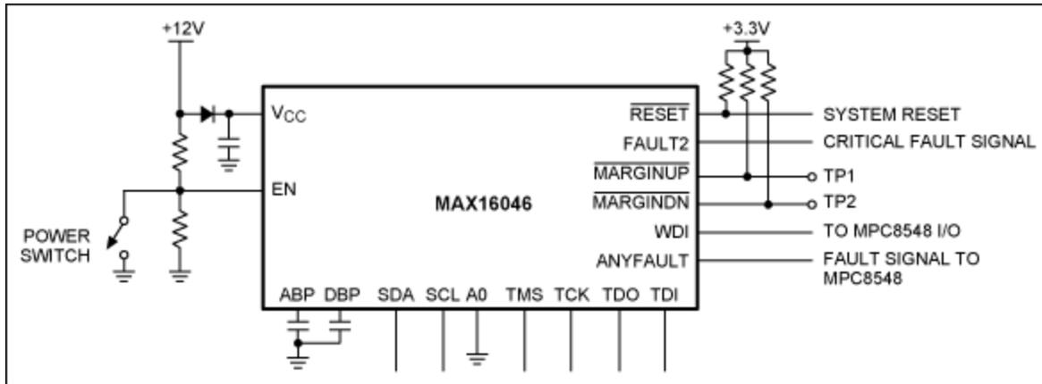
Figure 3. Detailed MAX16046 schematic.
