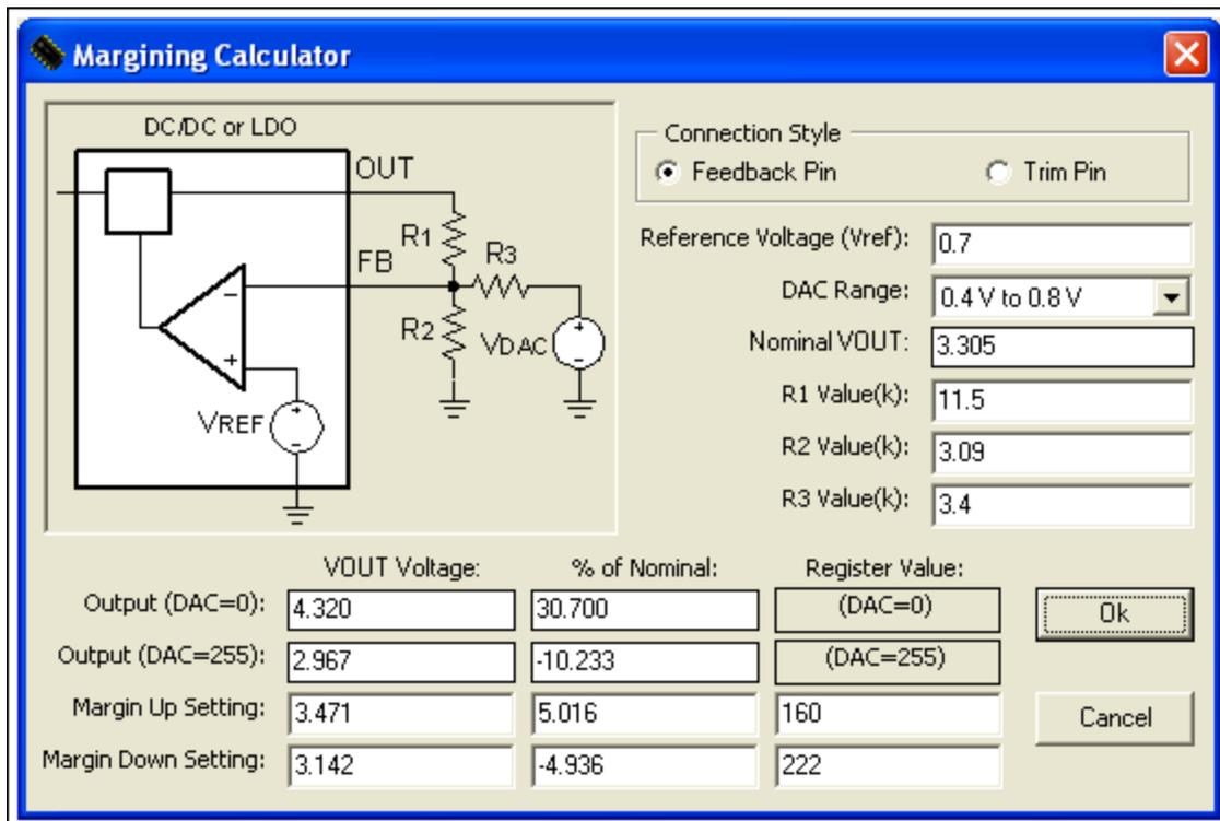
Figure 5. Margin calculator with parameters for 3.3V rail.
