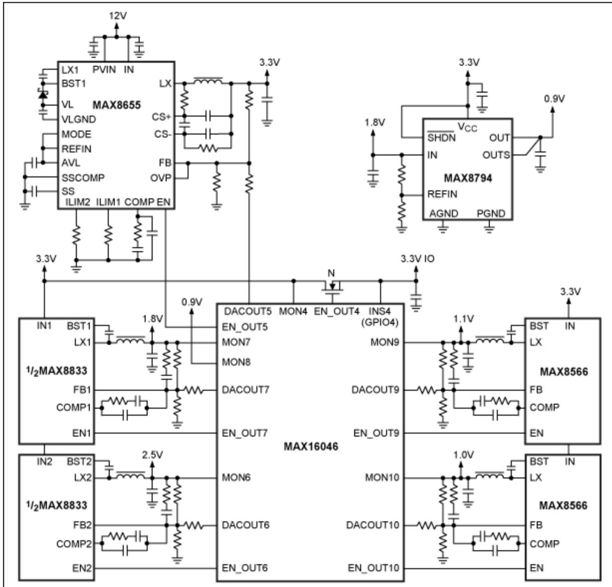
Figure 2. Partial schematic diagram with MAX16046.
