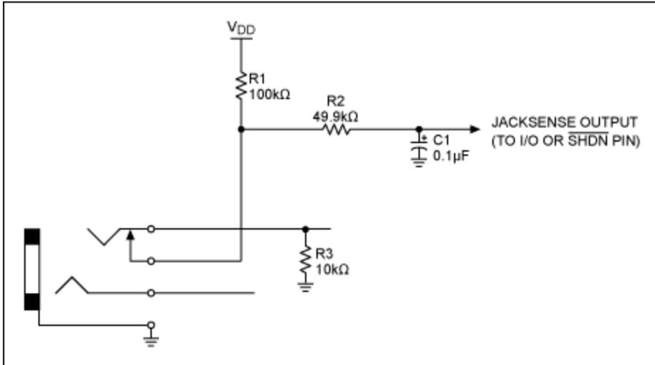
Figure 1. Jack-sensing circuit.
