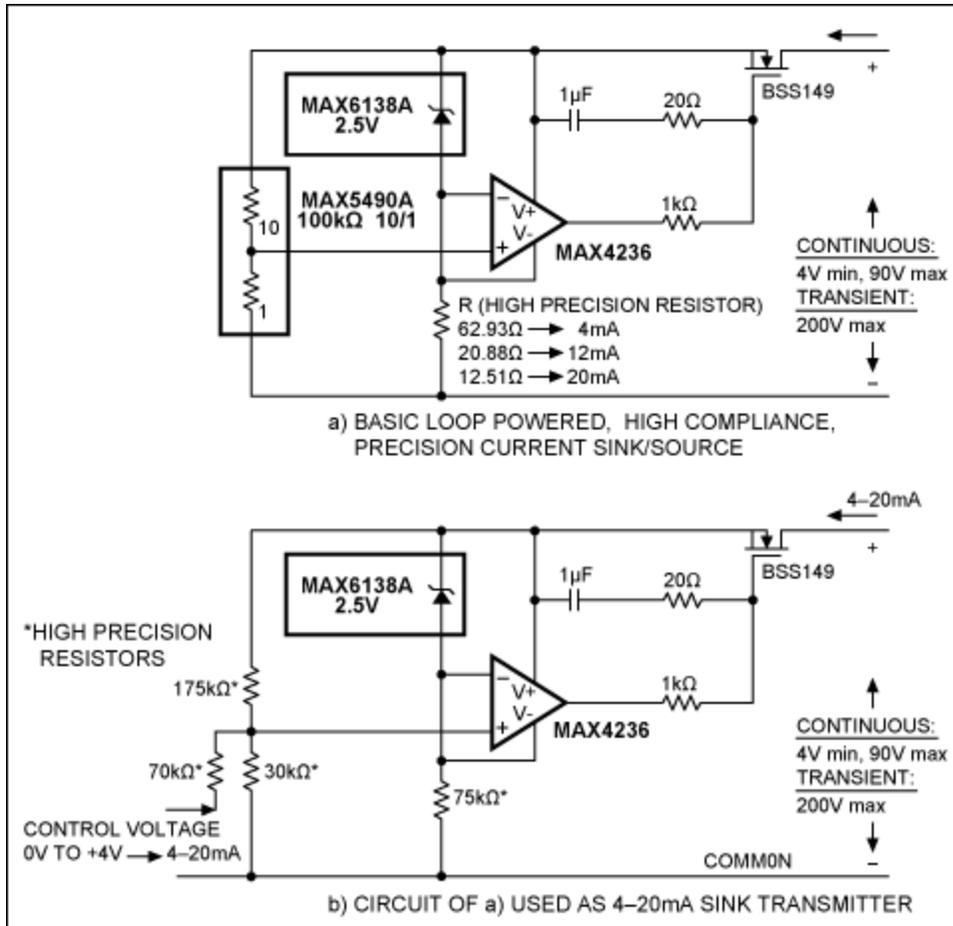
Figure 1. This basic loop-powered, high-compliance, precision current sink (or source) (a) can be modified for use as a 4-20mA sink transmitter (b).
