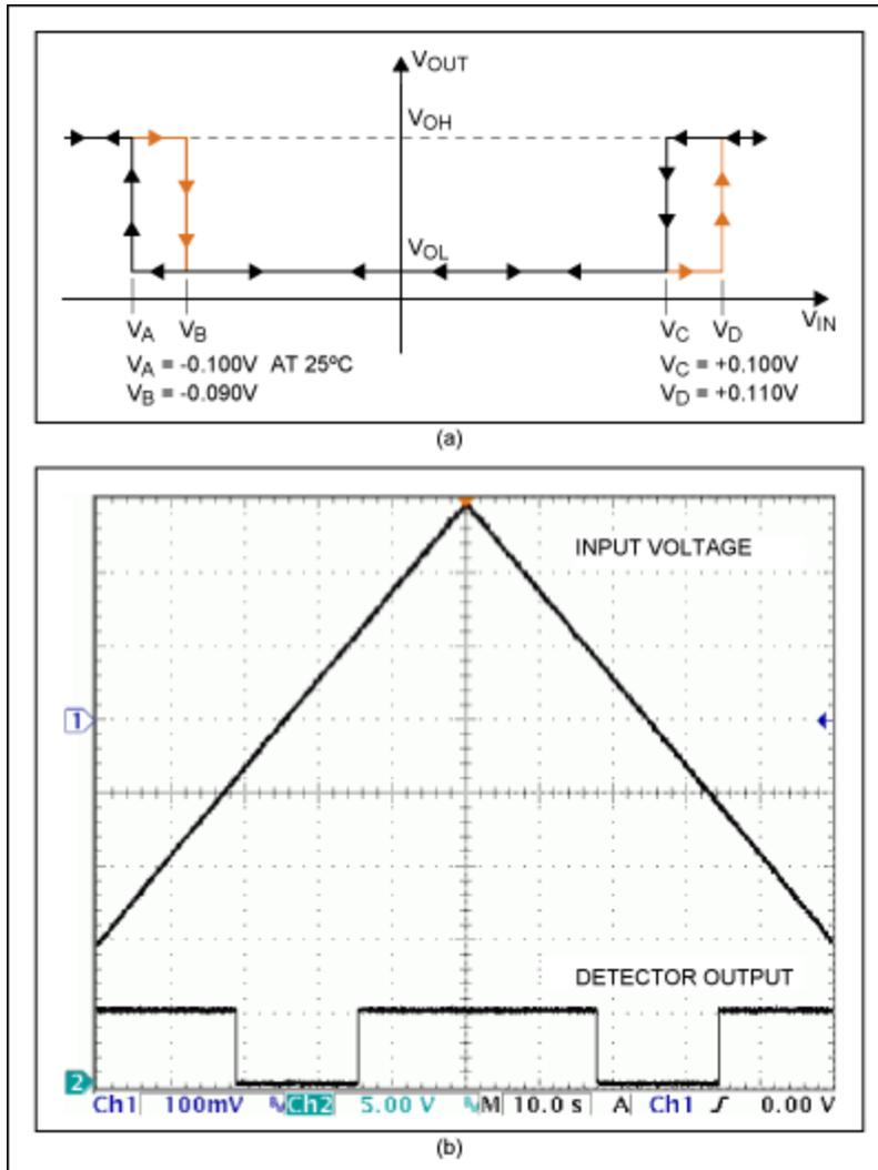
Figure 2. These waveforms from the Figure 1 circuit show the response of the detector output to an input-voltage ramp.
