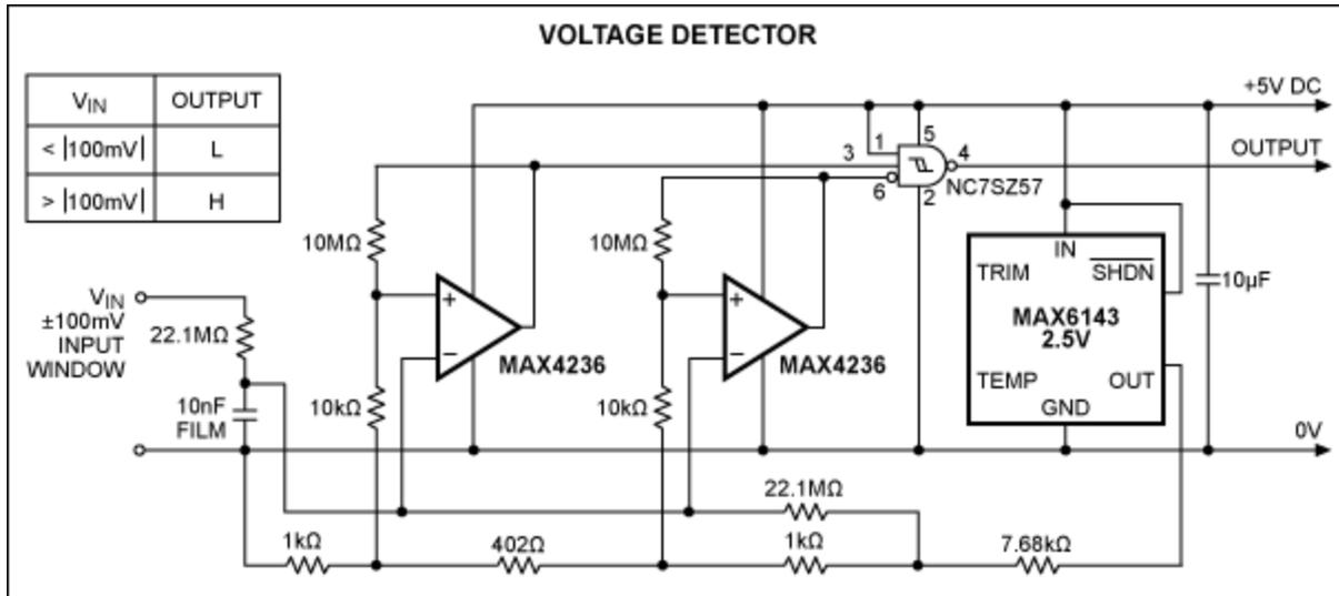
Figure 1. This detector of bipolar DC voltages asserts a digital output signal when the input is within a  $\pm 100\text{mV}$  window, centered at  $0\text{V}$ .
