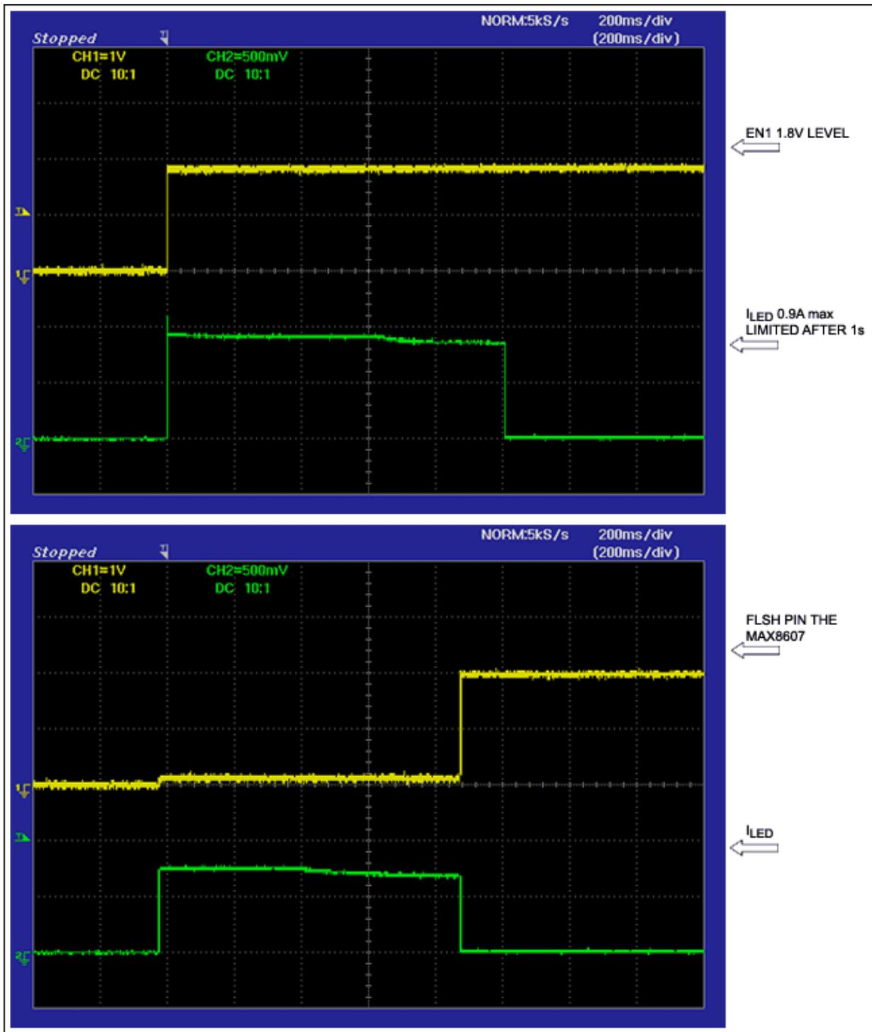
Figure 2. When EN1 goes high, the timeout period of the reset circuit is initiated and when timeout occurs it reduces the LED current by bringing its reset output high (top). When the Flash pin on the MAX8607 goes high, current to the LED is reduced, thus preventing overheating (bottom).
