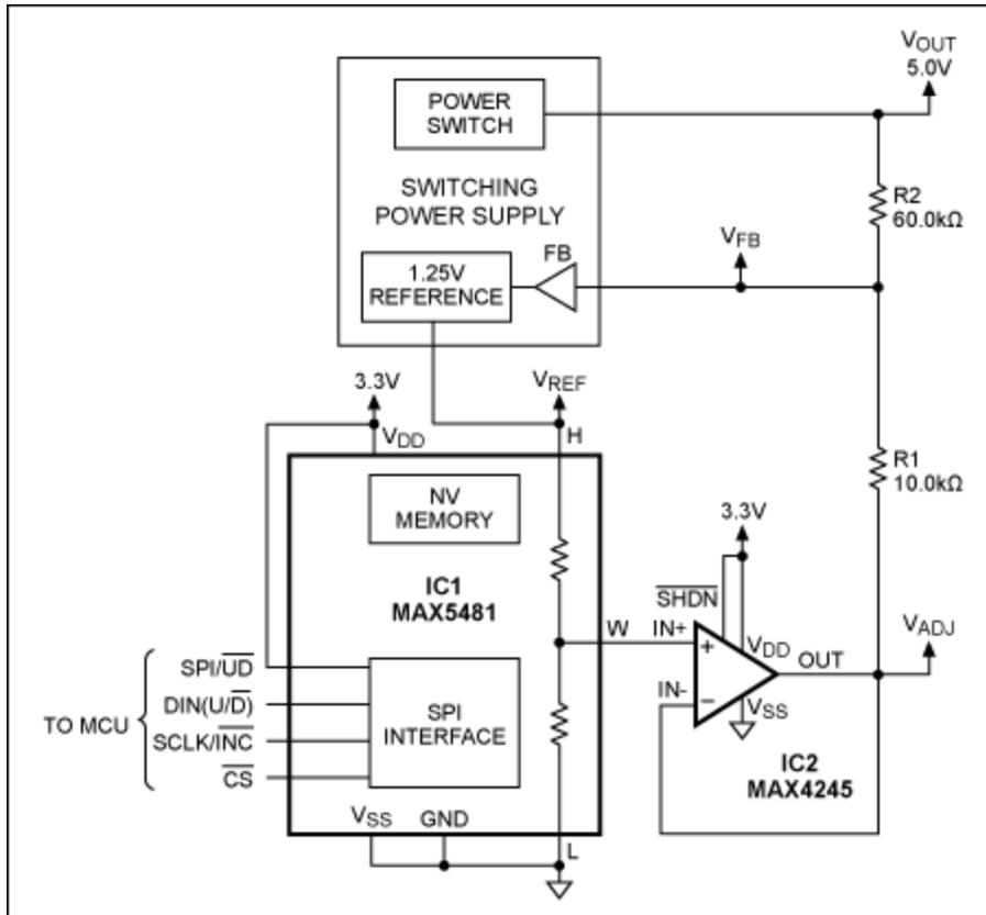
Figure 1. By introducing a solid-state potentiometer (IC1) and buffer amplifier as shown, you can digitally control the power supply's output voltage via a serial data link.
