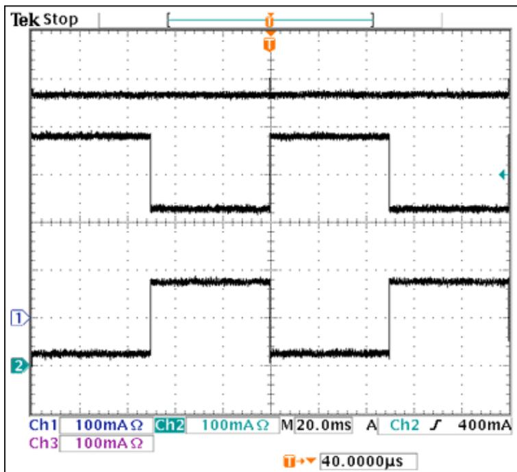
Figure 3. These waveforms from the Figure 2 circuit show that the sum of the essential-circuitry current (middle trace) and storage-element current (bottom trace) is always less than the 500mA maximum specified
