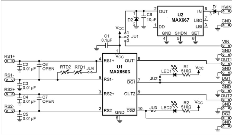
Figure 2. MAX6603EVKIT schematic.
