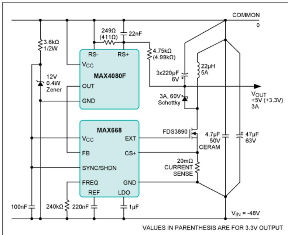
Figure 1. This simple power converter derives +5V (or +3.3V) from -48V.
