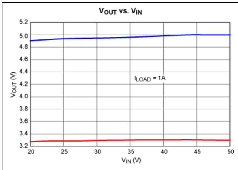
Figure 2.  $V_{OUT}$  vs.  $V_{IN}$  for the circuit in Figure 1. Graph shows that circuit regulation at a constant load of 1A improves somewhat for the higher input voltages for both the +5V and +3.3V versions.
