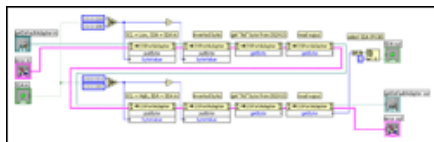
Figure 4. The VI "I 2 C clock" toggles SCL from low to high. SDA can be set or reset for "I 2 C write" actions and read for "I 2 C read" actions.
