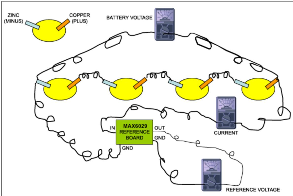
Figure 1. Lemon batteries running a voltage reference board.
