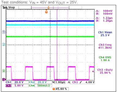
Ch1: output voltage; Ch2: input voltage; Ch3: MOSFET gate voltage; Ch4: output current.
