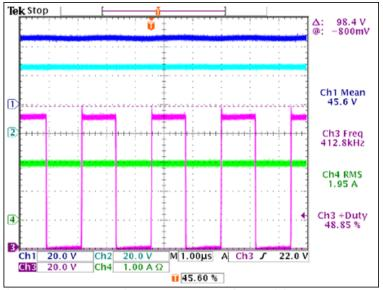
Ch1: output voltage; Ch2: input voltage; Ch3: MOSFET drain voltage; Ch4: output current.
