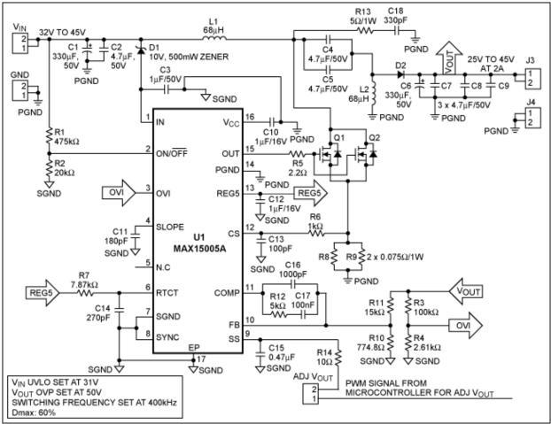
Figure 1. Schematic of the MAX15005A SEPIC converter for  $F_{SW} = 400 \text{kHz}$ .
