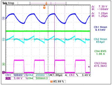
Ch1: output voltage; Ch2: input voltage; Ch3: MOSFET gate voltage; Ch4: output current.
