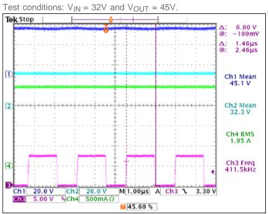
Ch1: output voltage; Ch2: input voltage; Ch3: MOSFET gate voltage; Ch4: output current.
