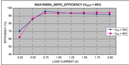
Figure 3. Load current vs. converter efficiency for  $V_{OUT} = 45V$ .
