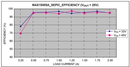
Figure 2. Load current vs. converter efficiency for  $V_{OUT} = 25V$ .
