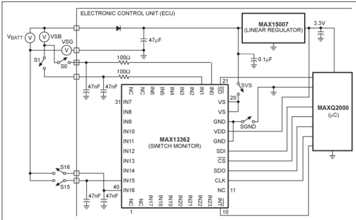
Figure 1. The MAX13362 test circuit.
