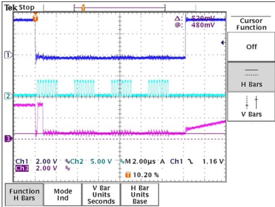
Figure 2. SPI readback shows ground shift. Ch1 = CS; Ch2 = CLK; Ch3 = SDO (data).
