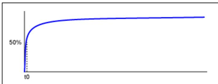
Figure 6. Step response of short/high-quality cable.
