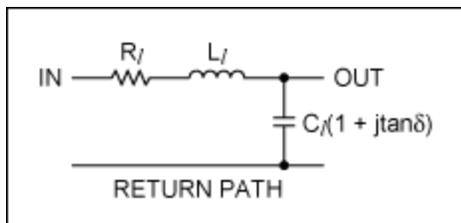
Figure 3. Simplified cable model.
