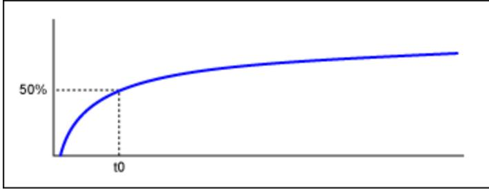
Figure 7. Step response of longer/low-quality cable.
