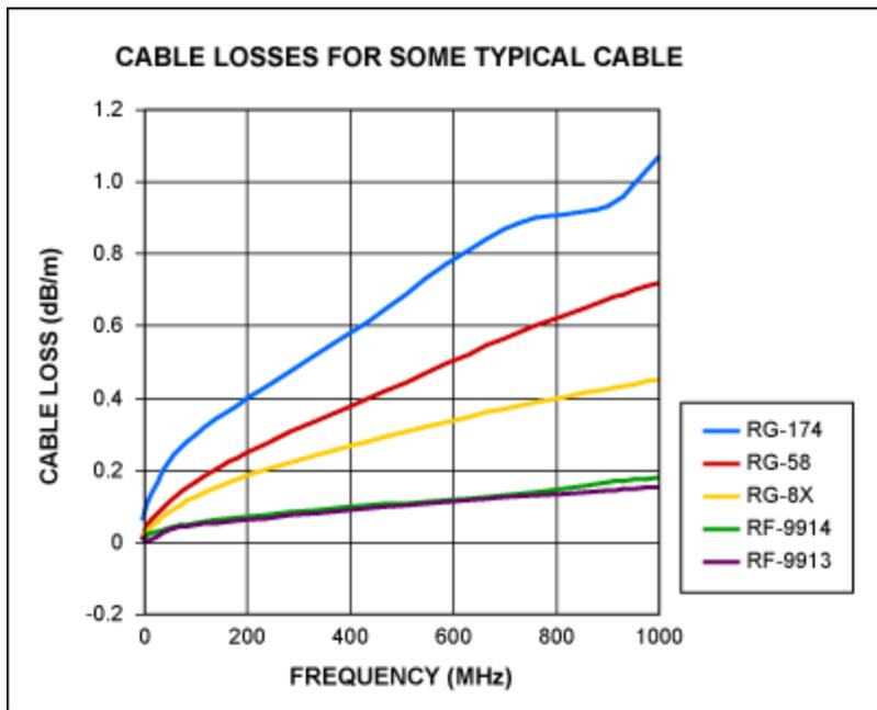
Figure 5. Cable losses for a variety of cables.
