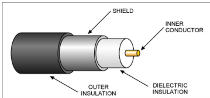
Figure 2. Typical coaxial cable.
