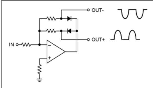
Figure 3. Diodes in the feedback path enable this op-amp circuit to perform full-wave rectification without the loss associated with forward-voltage drops in the diodes.
