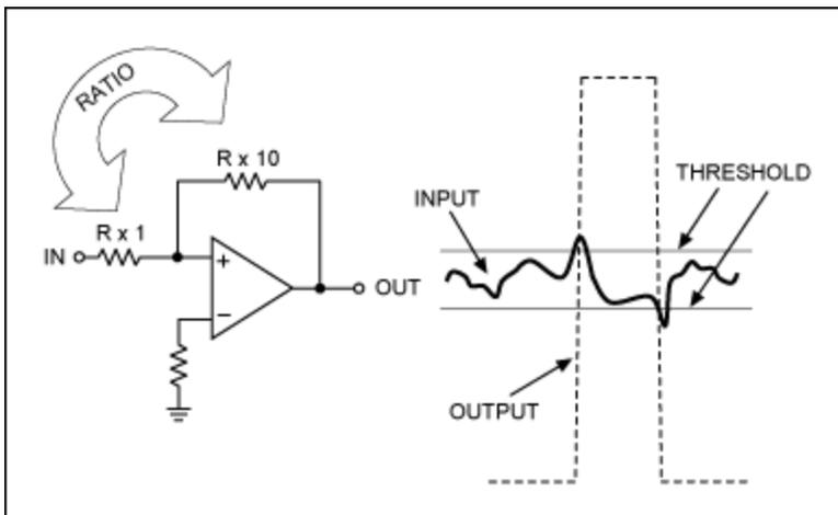
Figure 4. The modest bandwidth of this inexpensive op amp allows the Schmitt-trigger circuit to ignore high-frequency noise.
