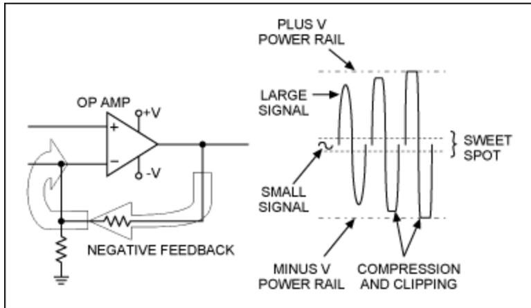
Figure 1. Signal conditions determine the bandwidth through an op amp.
