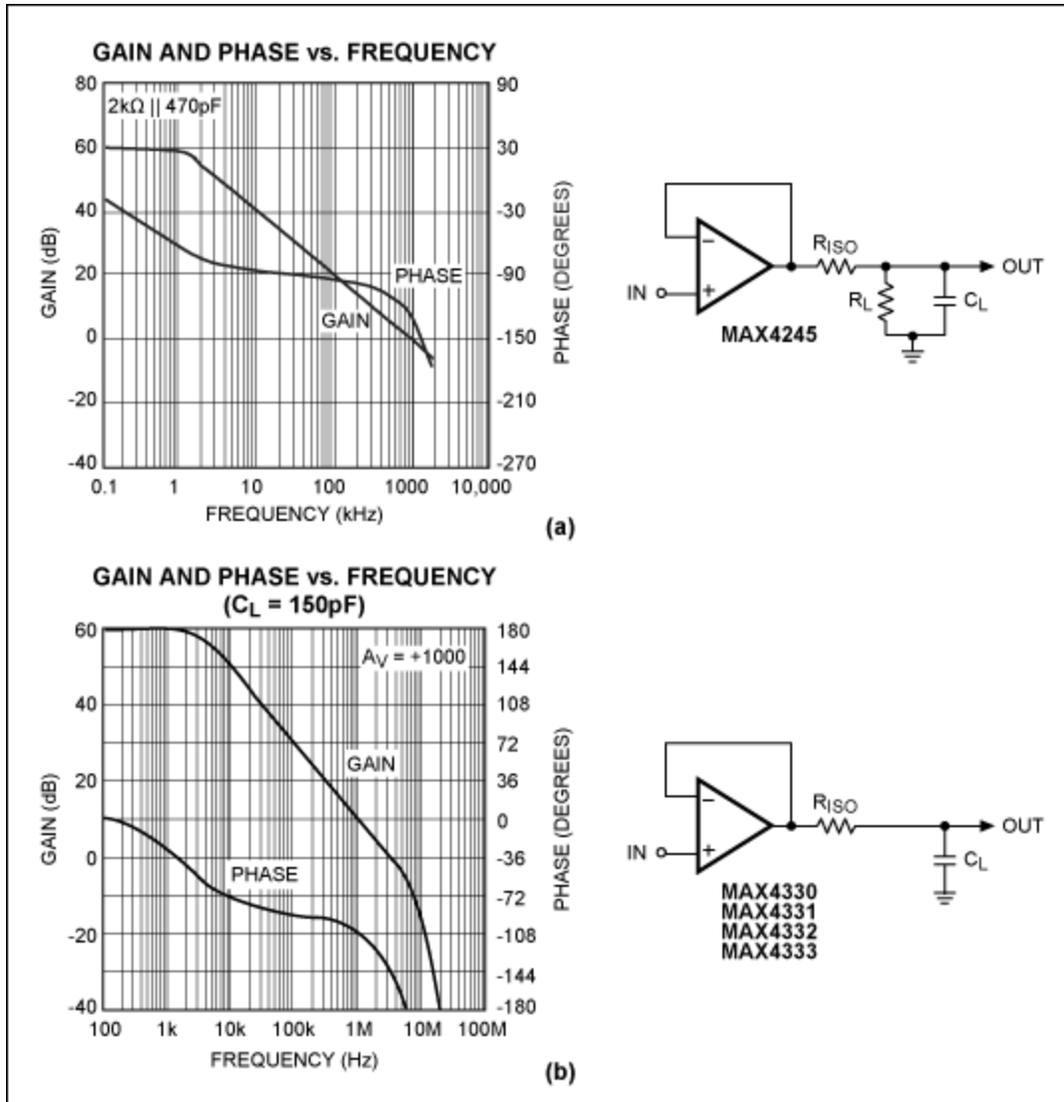
Figure 2. These circuits operate with inexpensive op amps because they deliberately limit the signal bandwidth to 1MHz (a), and 3MHz (b).
