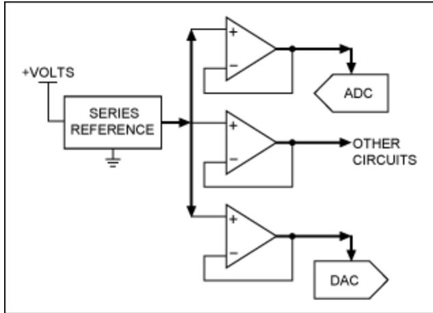
Figure 5. These inexpensive op amps distribute a single reference voltage to various circuits, while their low bandwidth serves as a welcome noise filter.
