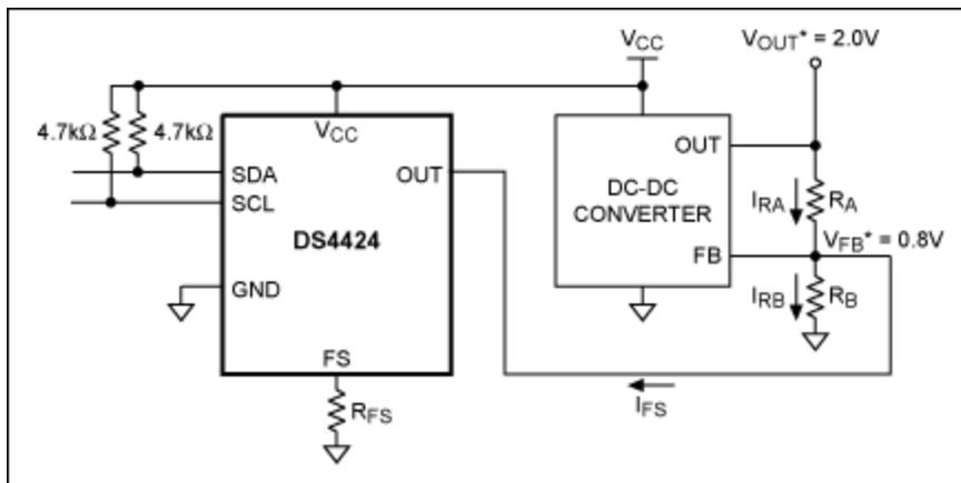
Figure 1. DC-DC converter circuit with adjustable-current DACs used to margin the converter's output voltage. \* $V_{OUT}$  and  $V_{FB}$  values are determined by the DC-DC converter, and should not be confused with  $V_{OUT}$  and  $V_{RFS}$  of the DS4424.
