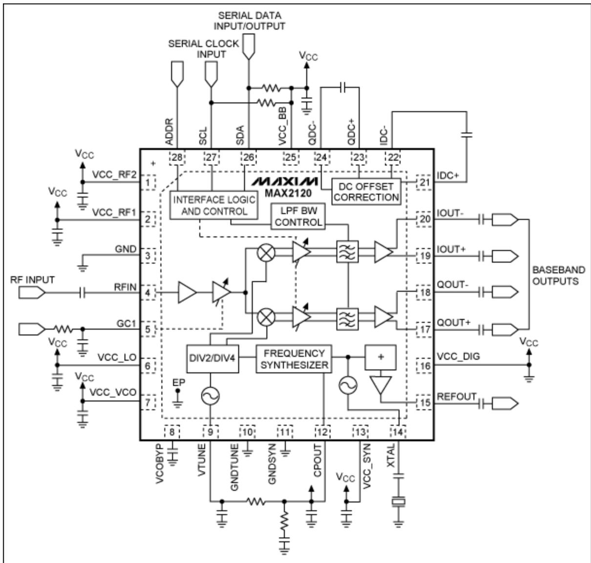
Figure 1. Typical operating circuit.
