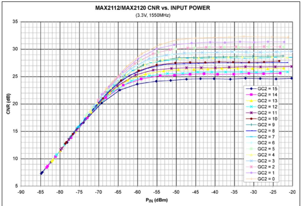
Figure 12. CNR vs. input power.
