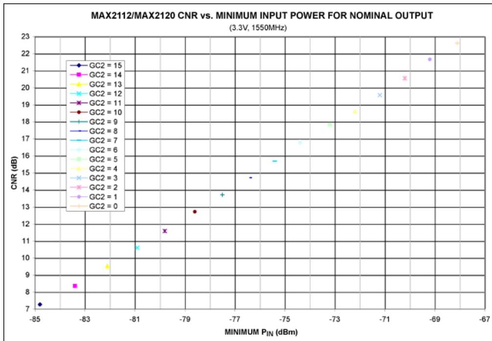
Figure 14. CNR vs. minimum input power (P<sub>IN</sub>).
