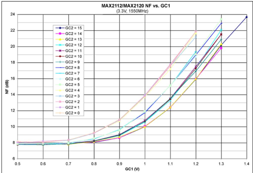
Figure 9. NF vs. GC1 voltage.
