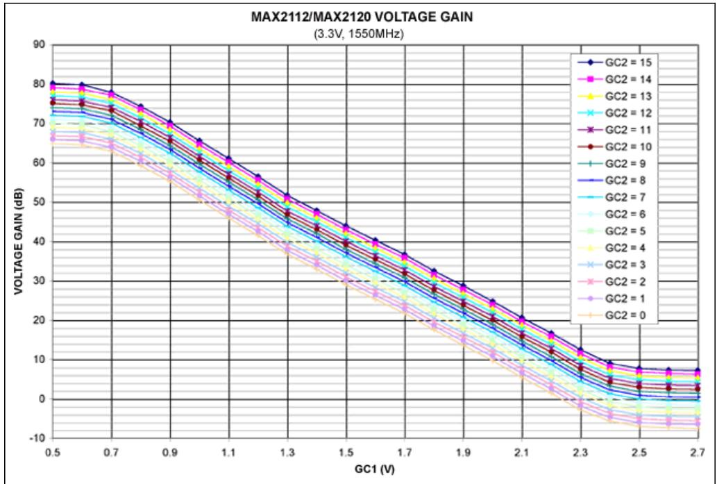
Figure 2. Voltage gain vs. GC1 voltage.
