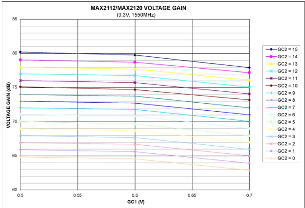
Figure 3. Voltage gain vs. GC1 voltage (zoomed scale).
