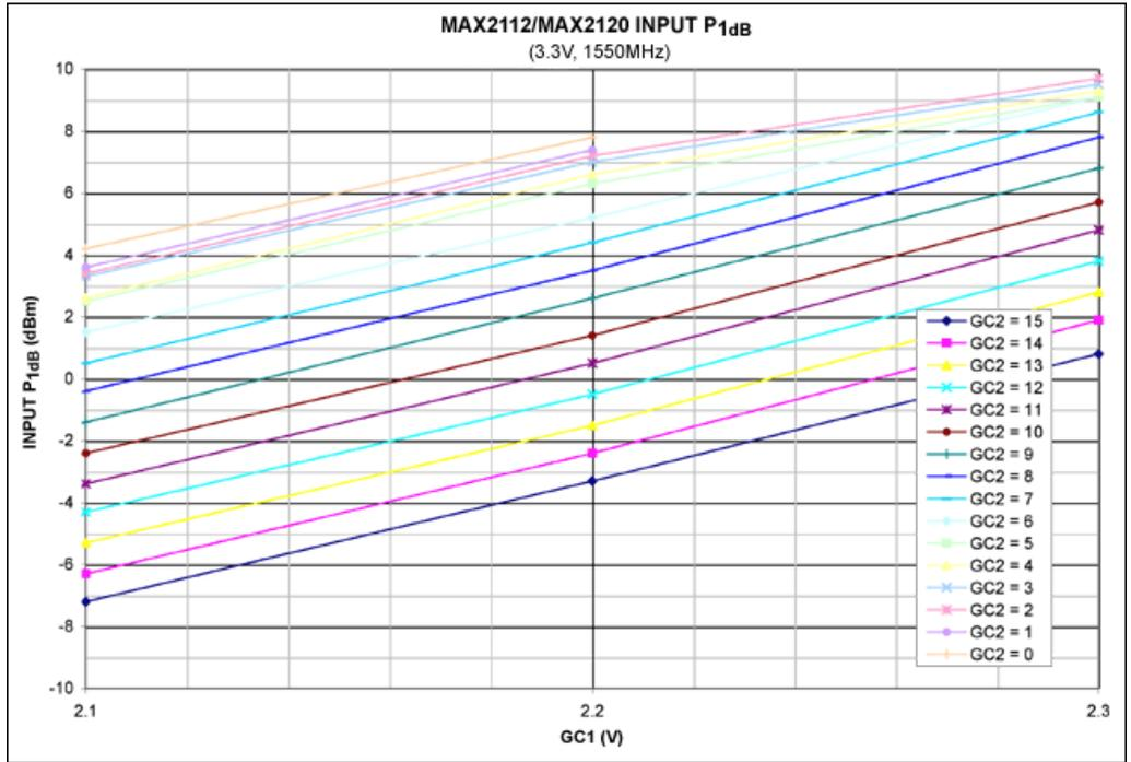
Figure 6. Input P<sub>1dB</sub> vs. GC1 voltage (zoomed scale).
