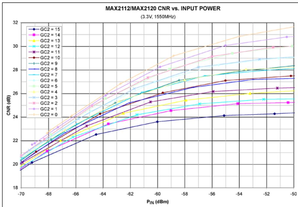
Figure 13. CNR vs. input power (zoomed scale).
