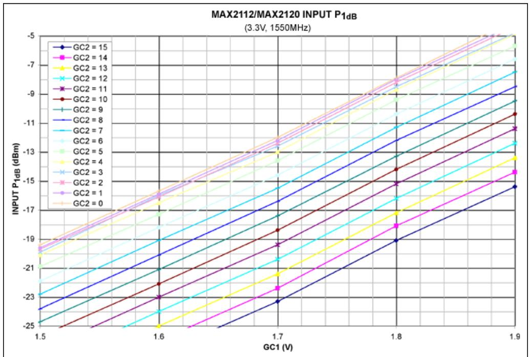
Figure 7. Input P<sub>1dB</sub> vs. GC1 voltage (zoomed scale).
