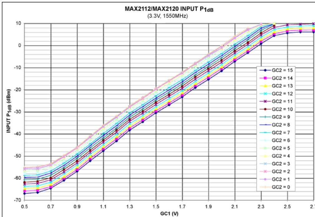
Figure 5. Input P<sub>1dB</sub> vs. GC1 voltage.
