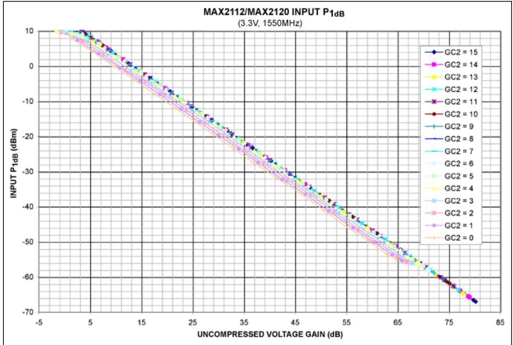
Figure 8. Input P<sub>1dB</sub> vs. uncompressed voltage gain.
