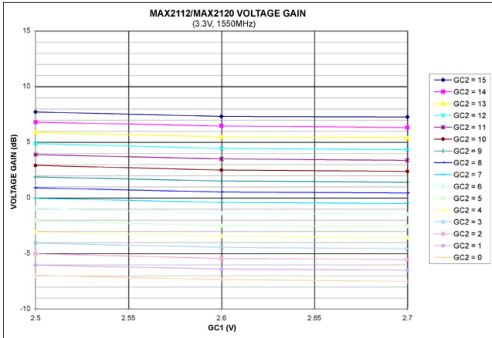
Figure 4. Voltage gain vs. GC1 voltage (zoomed scale).
