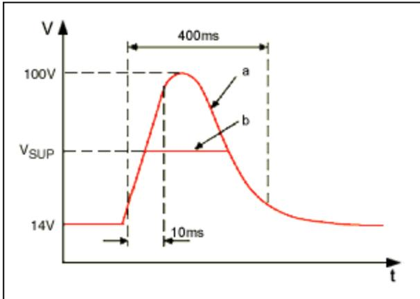
Figure 1. Typical load-dump surge shape: a) unsuppressed; b) suppressed.
