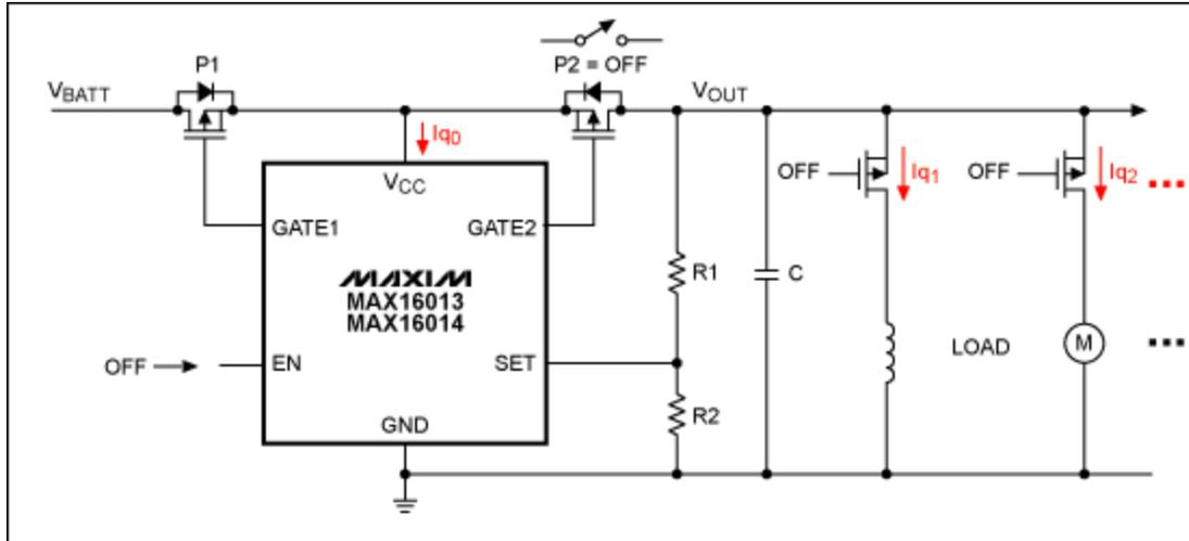
Figure 9. The MAX16013/MAX16014 are used as the main switch to reduce quiescent current consumption if an ECU is in OFF mode.
