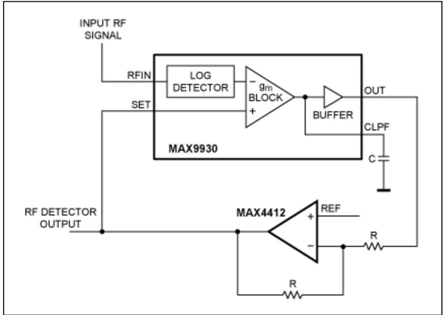
Figure 5. Used with the inverter MAX4412, the MAX9930 RF controller operates as a RF detector.
