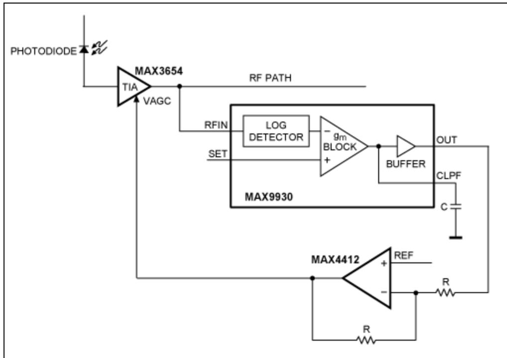
Figure 4. The MAX9930 is used in its typical application as a RF controller.
