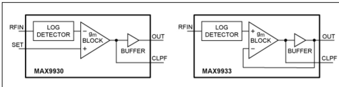
Figure 3. Block diagram of the MAX9930 (RF controller) and MAX9933 (RF detector).
