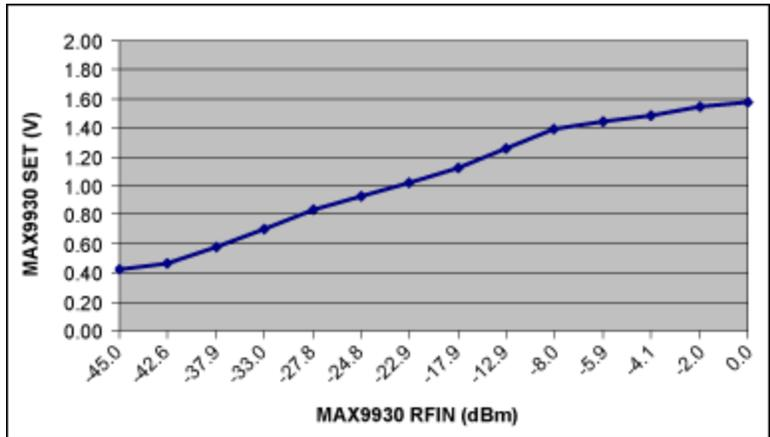
Figure 6. The relationship between SET vs. RFIN on the MAX9930 when it is used as a RF detector in the circuit of Figure 5.
