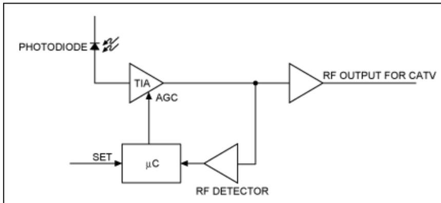
Figure 2. The TIA gain is adjusted with a digital feedback loop that involves a RF detector and a microcontroller.
