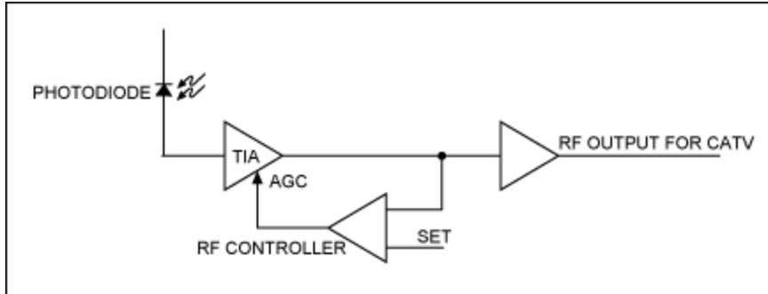
Figure 1. In a typical CATV application, the TIA gain is adjusted with an analog feedback loop by using a RF controller.
