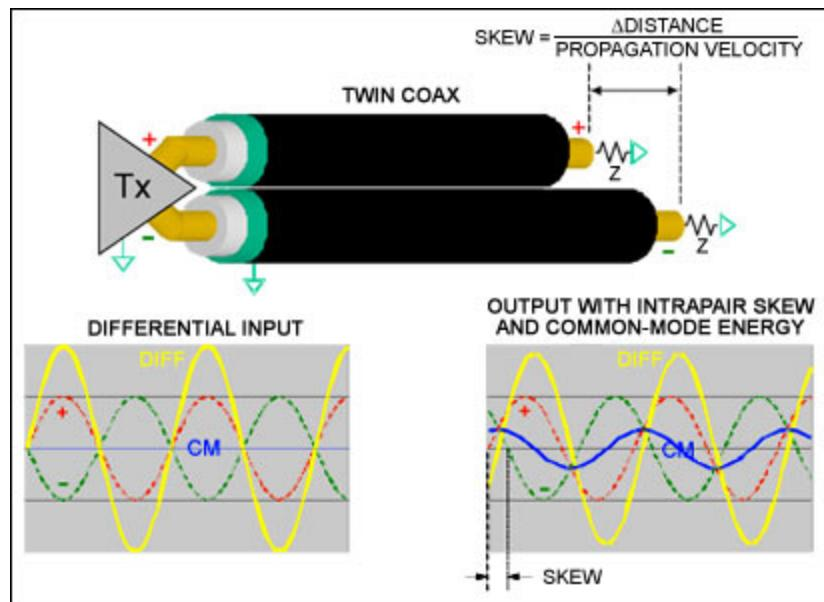
*Figure 1. Simple intrapair skew converts some differential signal to common-mode (CM) energy.*
