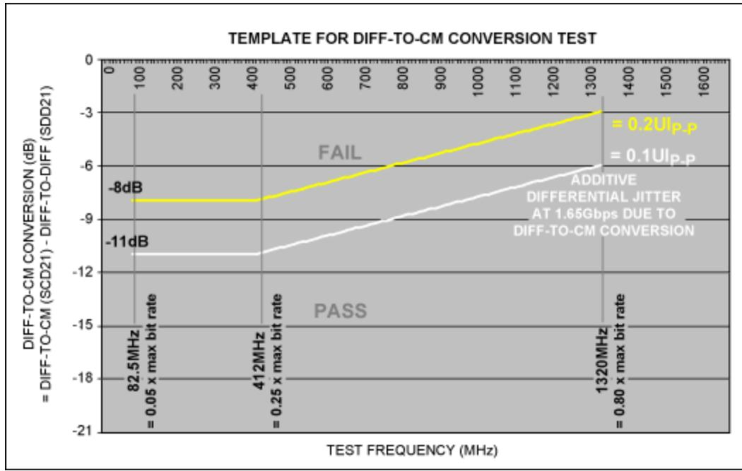
Figure 9. Simplified test template, for which  $0.1\text{UI}_{\text{P-P}}$  pass/fail criteria are recommended.
