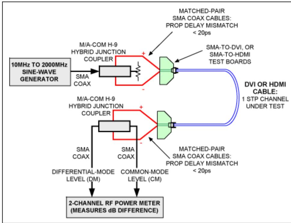
Figure 12. This test setup features a low-cost generator, couplers, and power meters.
