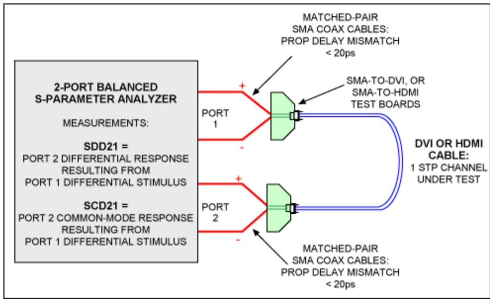
Figure 11. This 4-port S-parameter network analyzer is configured as a balanced 2-port analyzer.
