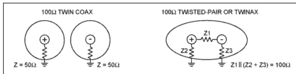
Figure 4. Uncoupled (twin coax) and coupled (twinax, STP)  $100\Omega$  differential pairs.
