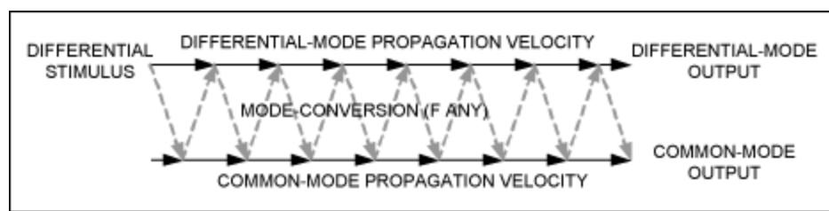
Figure 5. Illustration of mode conversion along cable length.
