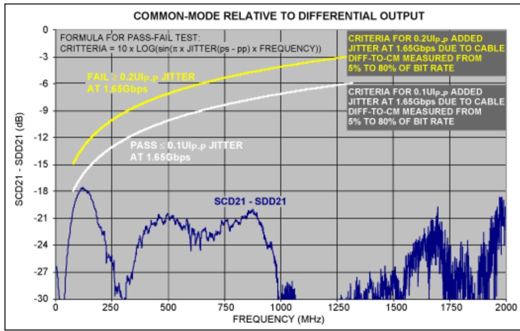
Figure 8. Plot of  $(SCD21 - SDD21)$  difference, with pass/fail template superimposed.
