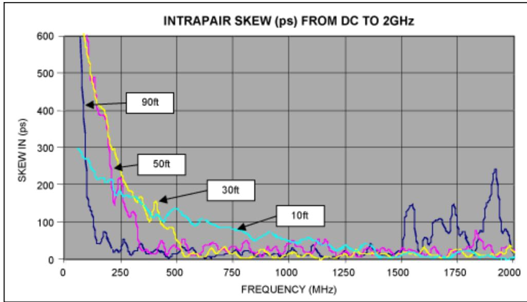
Figure 2. Intrapair skew vs. frequency for 28AWG twinax.
