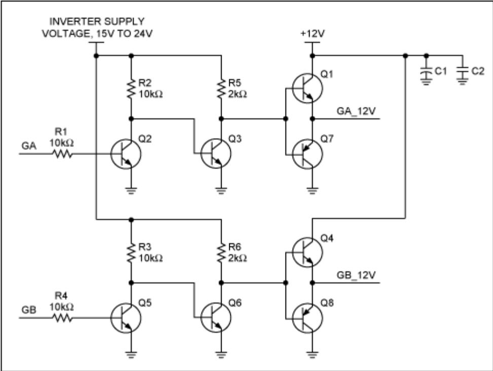
Figure 1. External circuitry required to enhance DS39xx gate-drive capacity.
