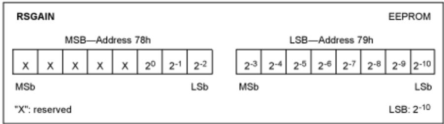
Figure 1. The calculated RSGAIN value should be written to addresses 78h and 79h using the above RSGAIN Register format.
