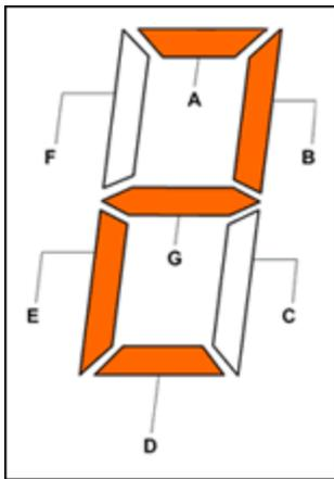
Figure 1. Seven-segment LCD display digit.
