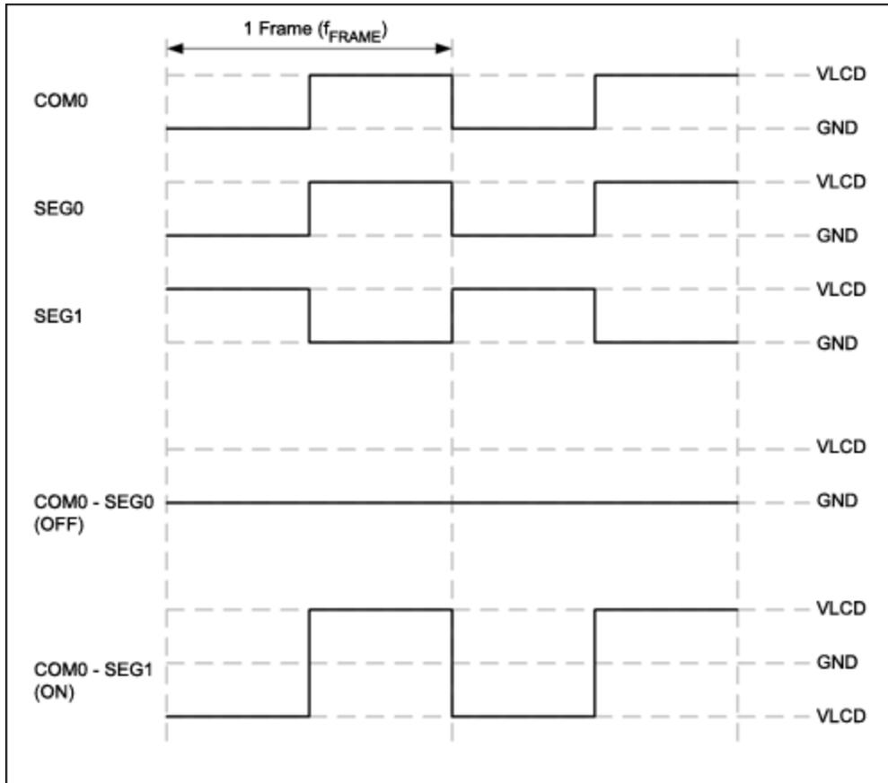
Figure 2. Alternating drive waveforms for static LCD segments.
