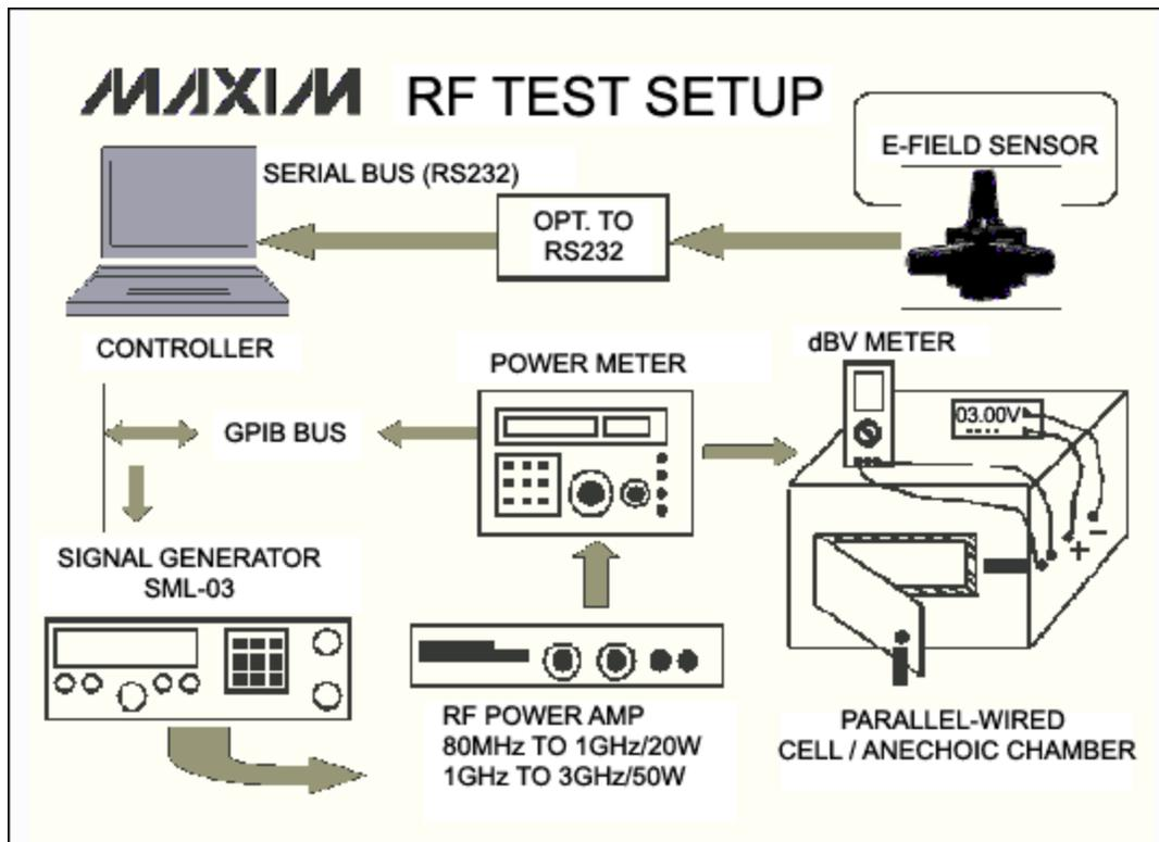
Figure 2. Equipment setup for RF noise-immunity testing.
