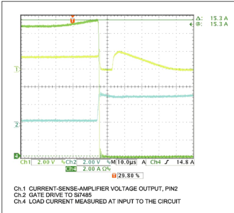
Figure 2. Test results for the Figure 1 circuit show an approximate response time of  $2\mu\text{s}$ .
