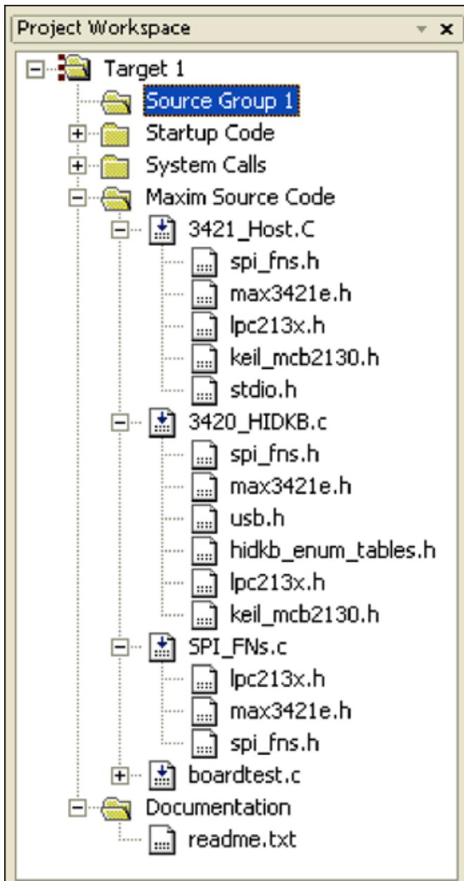
Figure 8. Structure of the Keil Project.
