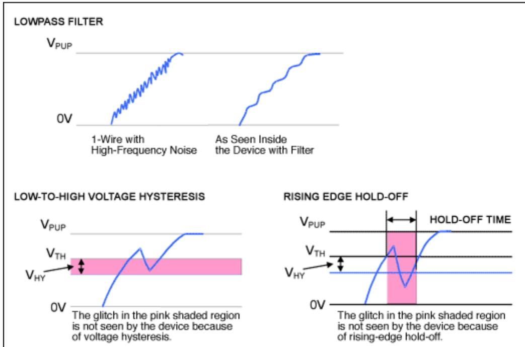
Figure 1. New 1-Wire front-end features.
