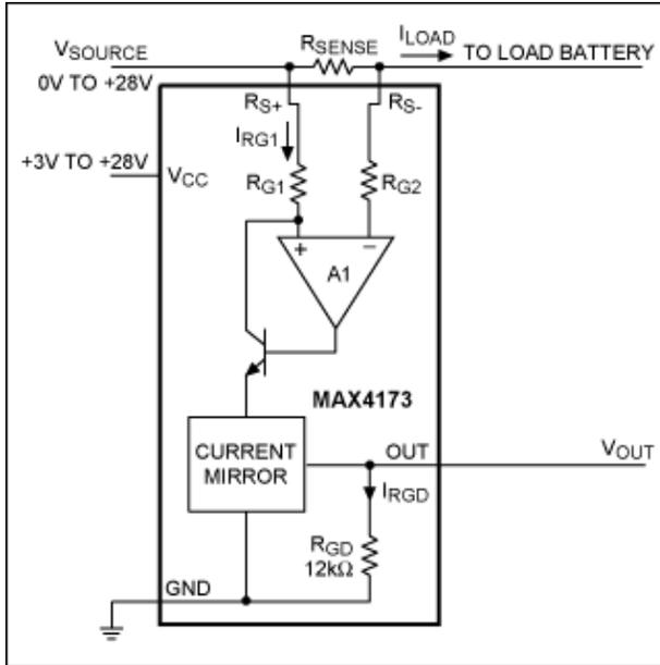
Figure 3. Internal functional diagram of the MAX4173.
