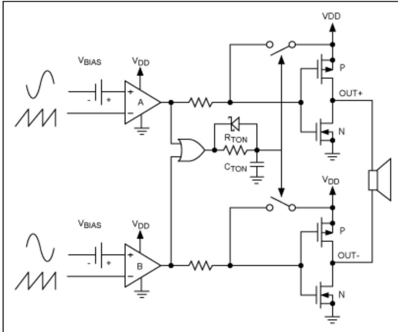
Figure 2. Mono Class D Amplifier Topology.
