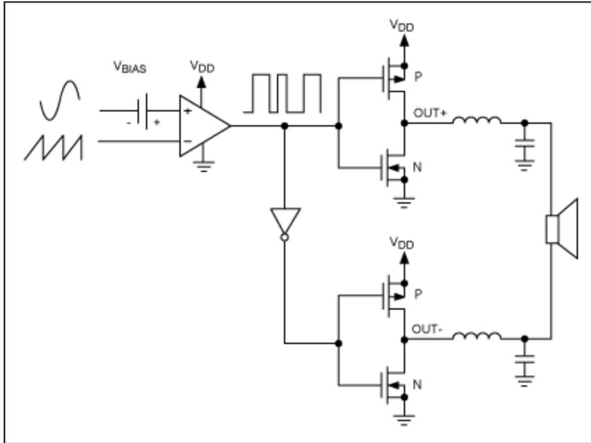
Figure 1. Conventional Pulse-Width-Modulation Topology.
