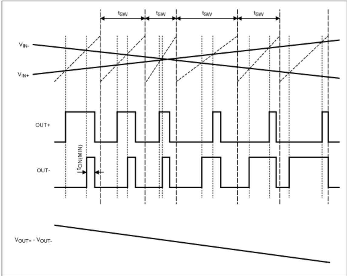
Figure 4. Maxim Class D BTL Output with Input Signal Applied, Spread-Spectrum-Modulation Mode.
