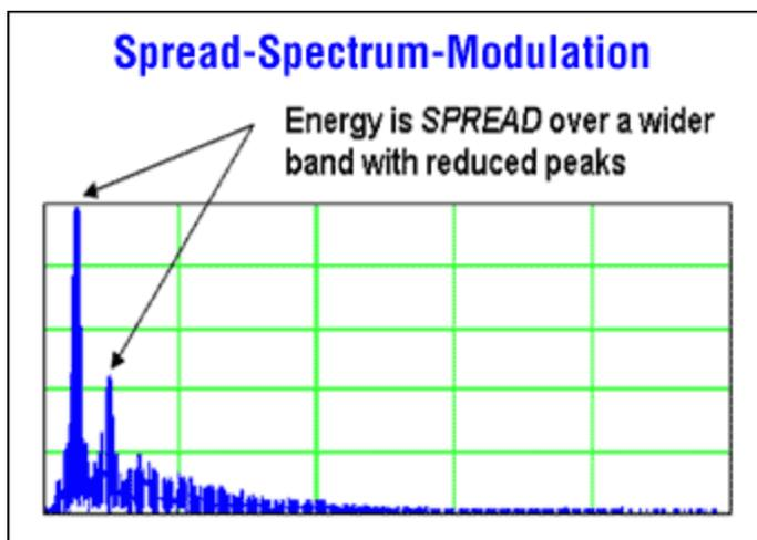
Figure 5b. Maxim's Spread-Spectrum-Modulation Mode.
