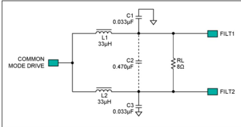
Figure 4. The traditional LC filter of Figure 3a looks like this to a common-mode signal.
