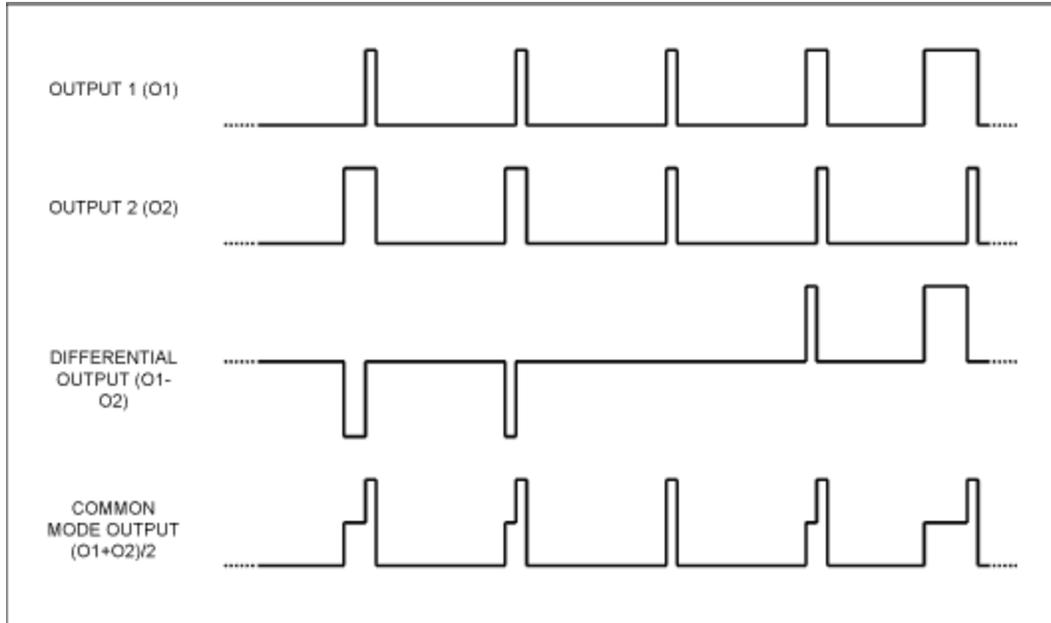
Figure 2. Modulation scheme for Maxim's MAX9704 stereo Class D amplifier.
