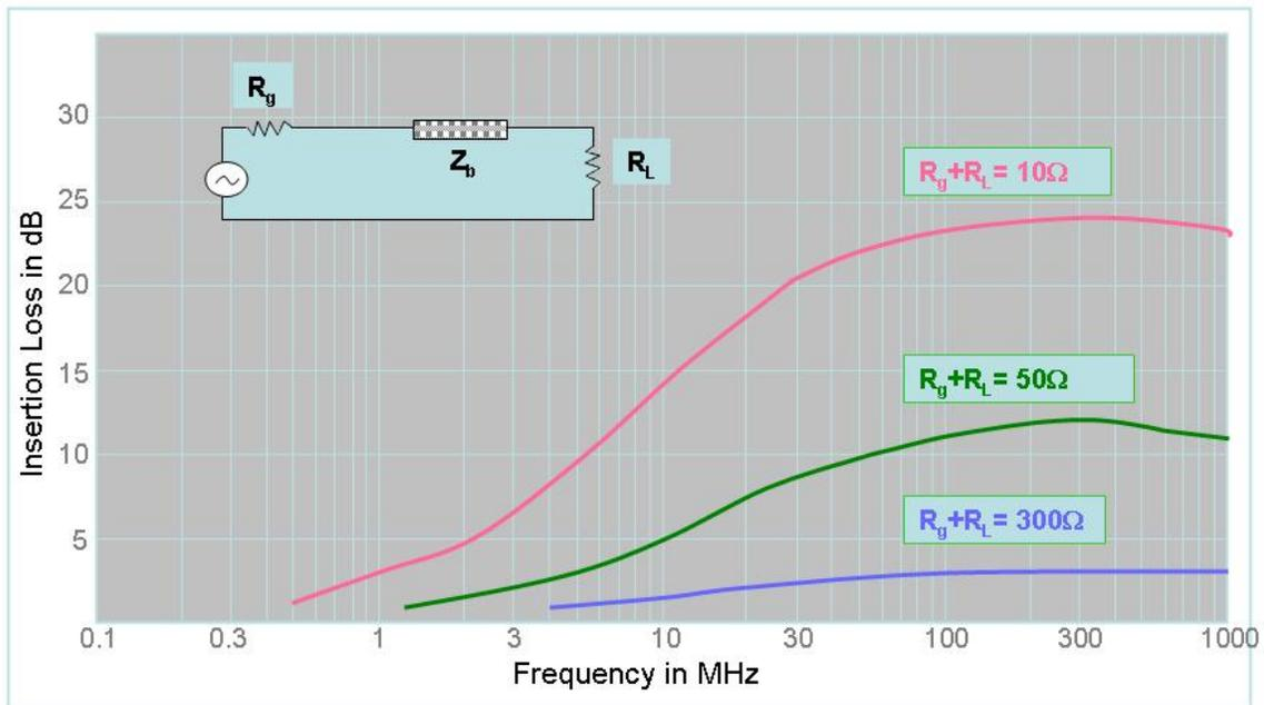
Figure 3. Bead insertion loss vs. frequency<sup>4</sup>.
