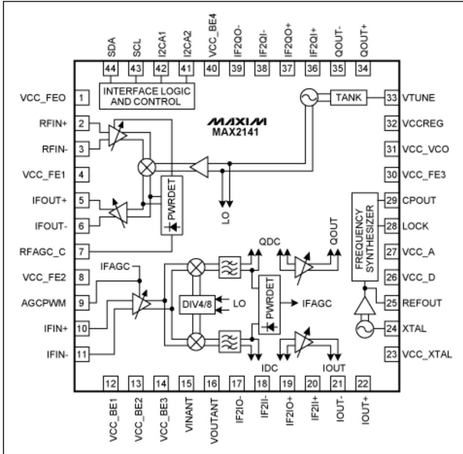
Figure 1. Schematic of the MAX2141 functional block diagram.
