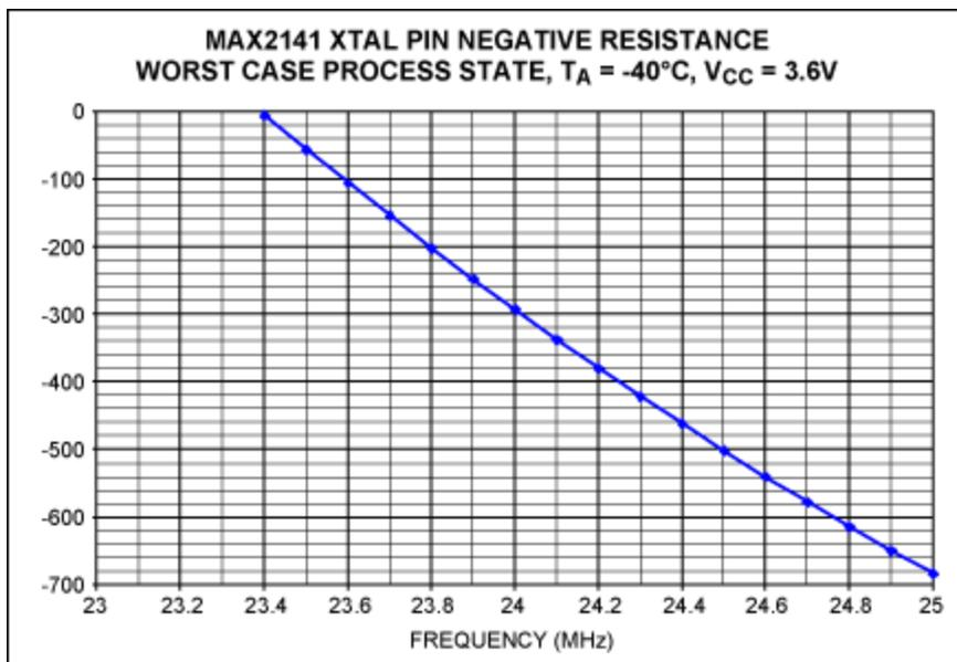
Figure 3. Simulated MAX2141 XTAL pin negative resistance for worst-case process, temperature, and supply voltage.
