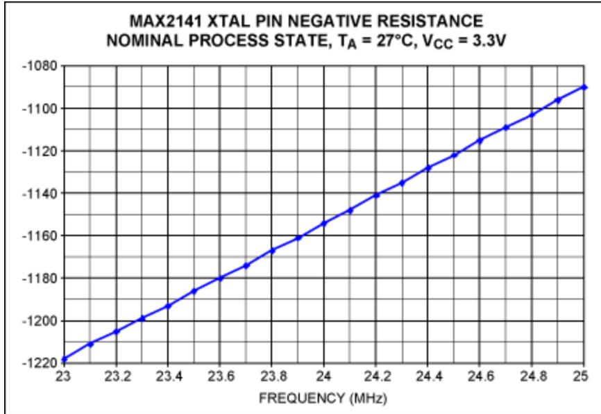
Figure 2. Simulated MAX2141 XTAL pin negative resistance for nominal process, temperature, and supply voltage.
