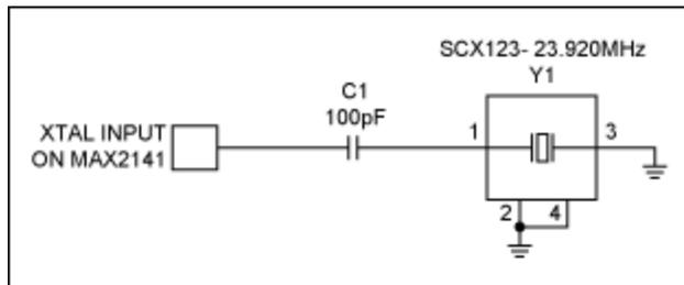
Figure 4. Typical external circuitry for the MAX2141 XTAL port.
