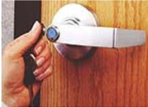
The iButton device is ideal for any application where information needs to travel with a person or object. Affixed to a key fob, watch, or ring, an iButton device can grant its owner access to a building, a PC, a piece of equipment, or a vehicle. Attached to a work tote, it can measure processes to improve efficiency, such as manufacturing, delivery, and maintenance. Some iButton devices can be used to store electronic cash for small transactions, such as
