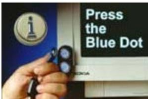
Information is transferred between your iButton device and a PC with a momentary contact at up to 142kbps. You simply touch your iButton device to a Blue Dot™ receptor or other iButton probe, which is connected to a PC. The Blue Dot receptor is cabled to a 1-Wire adapter that is attached to a spare PC port. 1-Wire adapters exist for USB, serial, and parallel ports. The Blue Dot receptor and 1-Wire adapter are inexpensive. See our [Maxim Direct](#)
