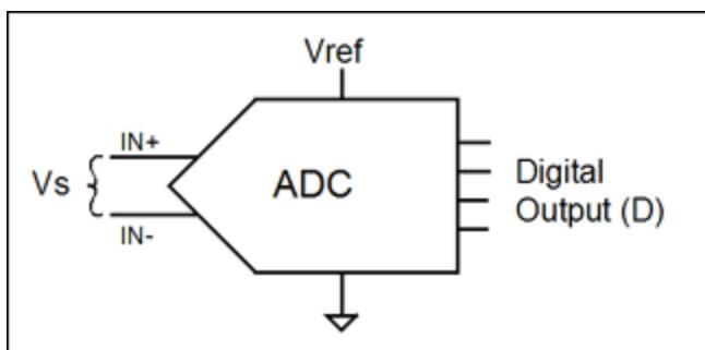
Figure 2. Generic analog-to-digital converter.
