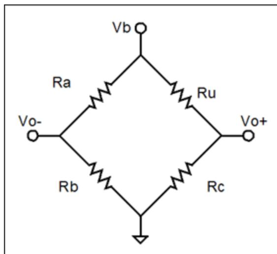
Figure 9. Illustration of a Wheatstone bridge which is comprised of two voltage-dividers powered from the same voltage source.
