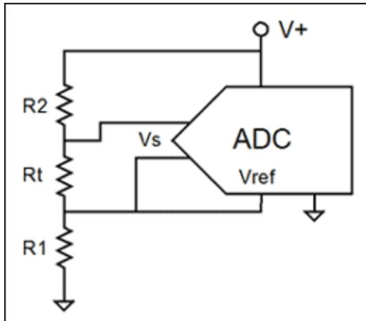
Figure 6. This circuit does not require a bridge or stable current source to measure  $R_t$ .
