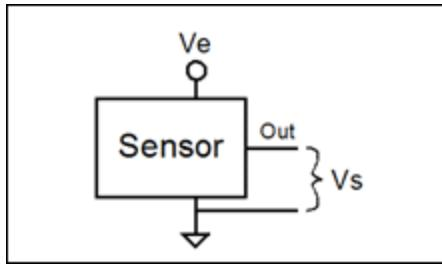
Figure 1. Generic ratiometric sensor.
