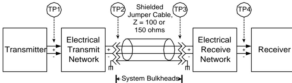
Figure 6. Serial link using shielded jumper cable
