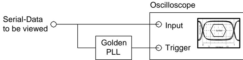
Figure 8. Viewing jitter using a sampling scope
