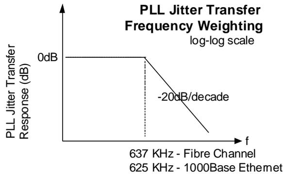
Figure 9. PLL jitter transfer using lowpass frequency weighting
