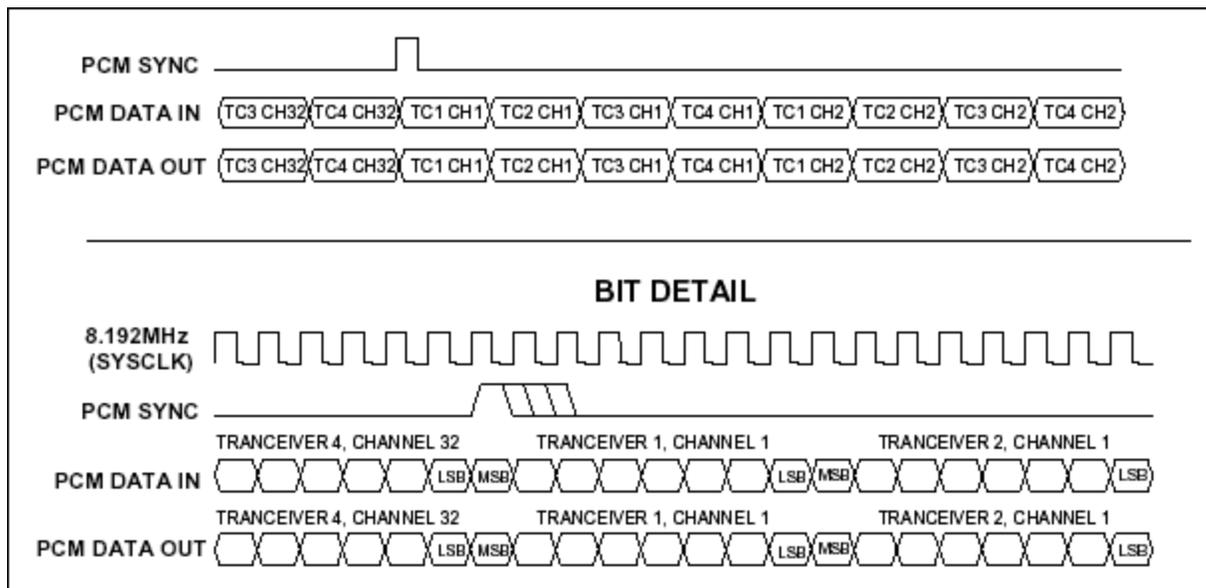
Figure 2. PCM Bus functional timing diagram.
