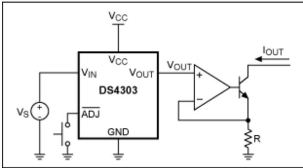
Figure 2. A simple circuit to realize a precise current sink using a DS4303 and several inexpensive components.
