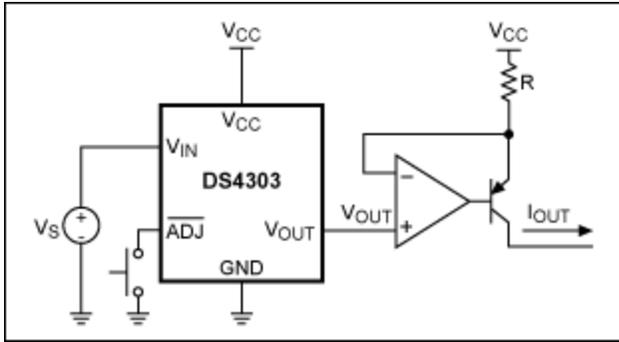
Figure 1. A simple circuit to realize a precise current source using a DS4303 and several inexpensive components.
