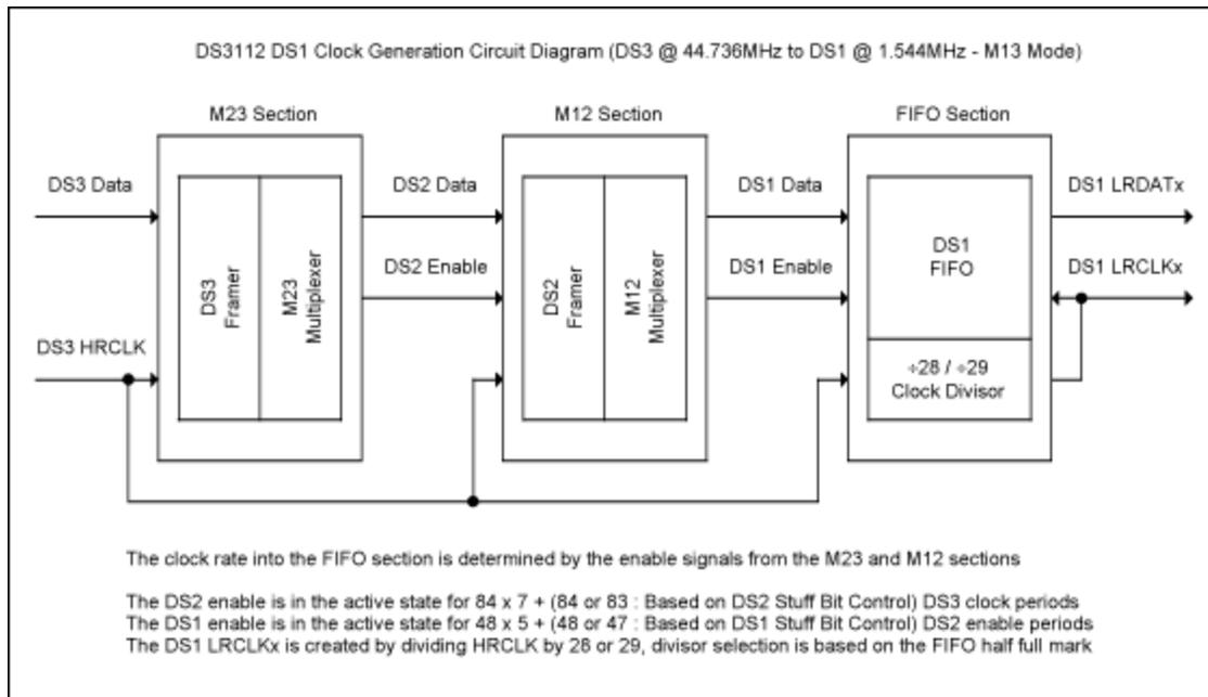
Figure 1. M13 and C-Bit parity modes.
