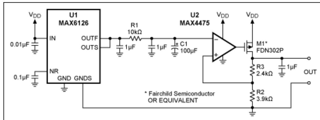
Figure 1. This ultra-low-noise LDO, the MAX6126, combines low-noise components with filtering to achieve an output noise floor of 6nV/ $\sqrt{\text{Hz}}$ .
