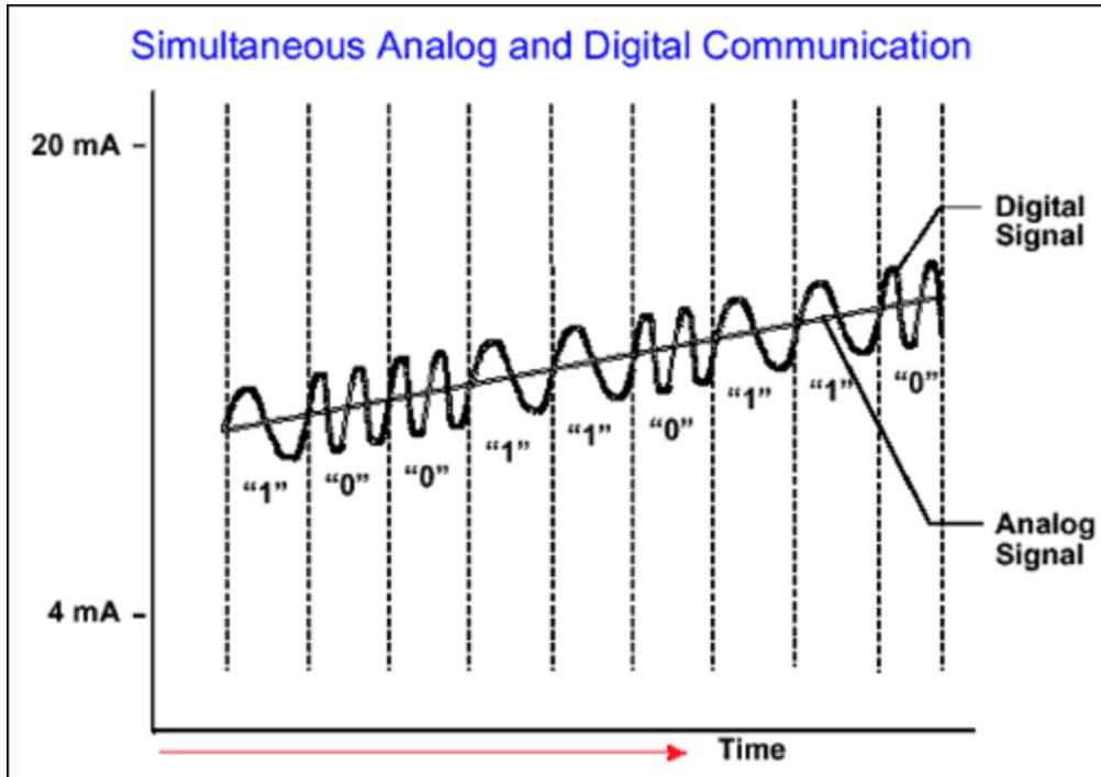
Figure 3. Simultaneous analog and digital communications.
