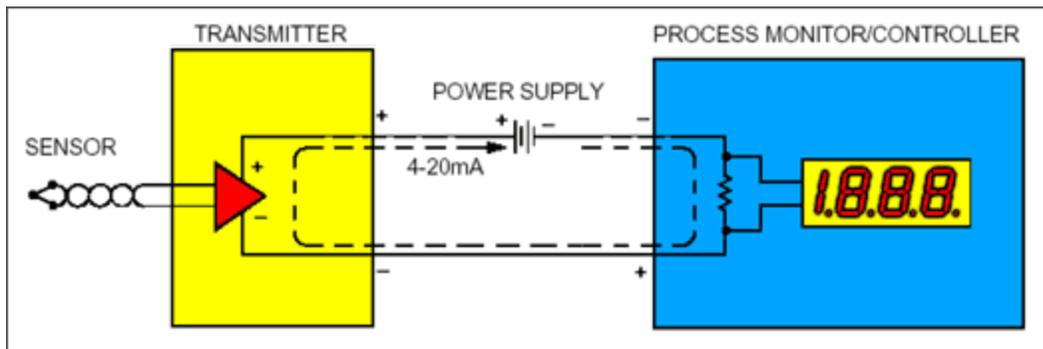
Figure 1. Diagram of a 4-20mA loop-powered circuit.
