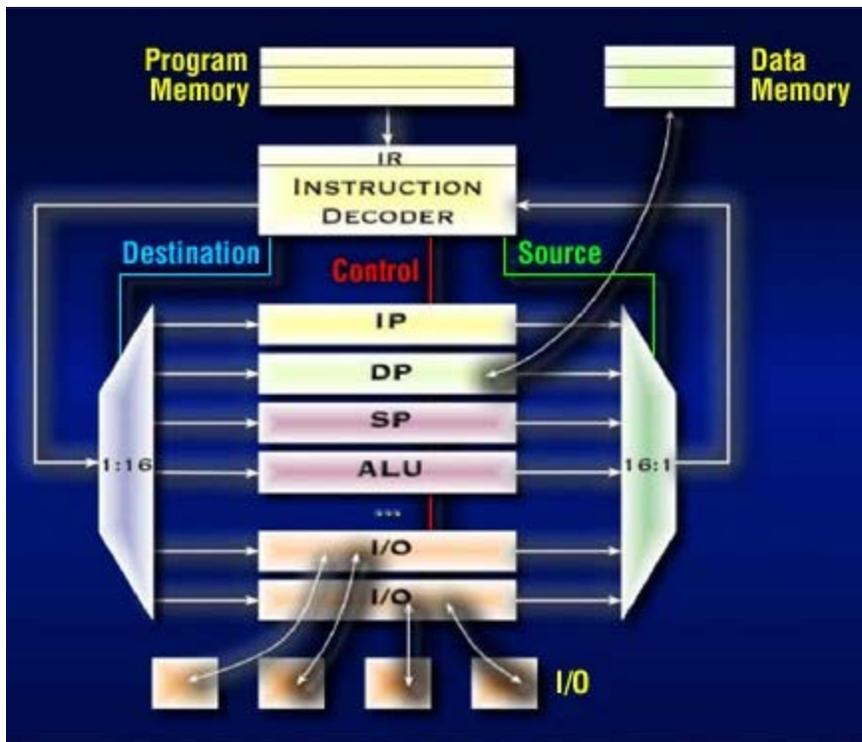
Figure 4. Illustration of the MAXQ  $\mu$ C architecture.
