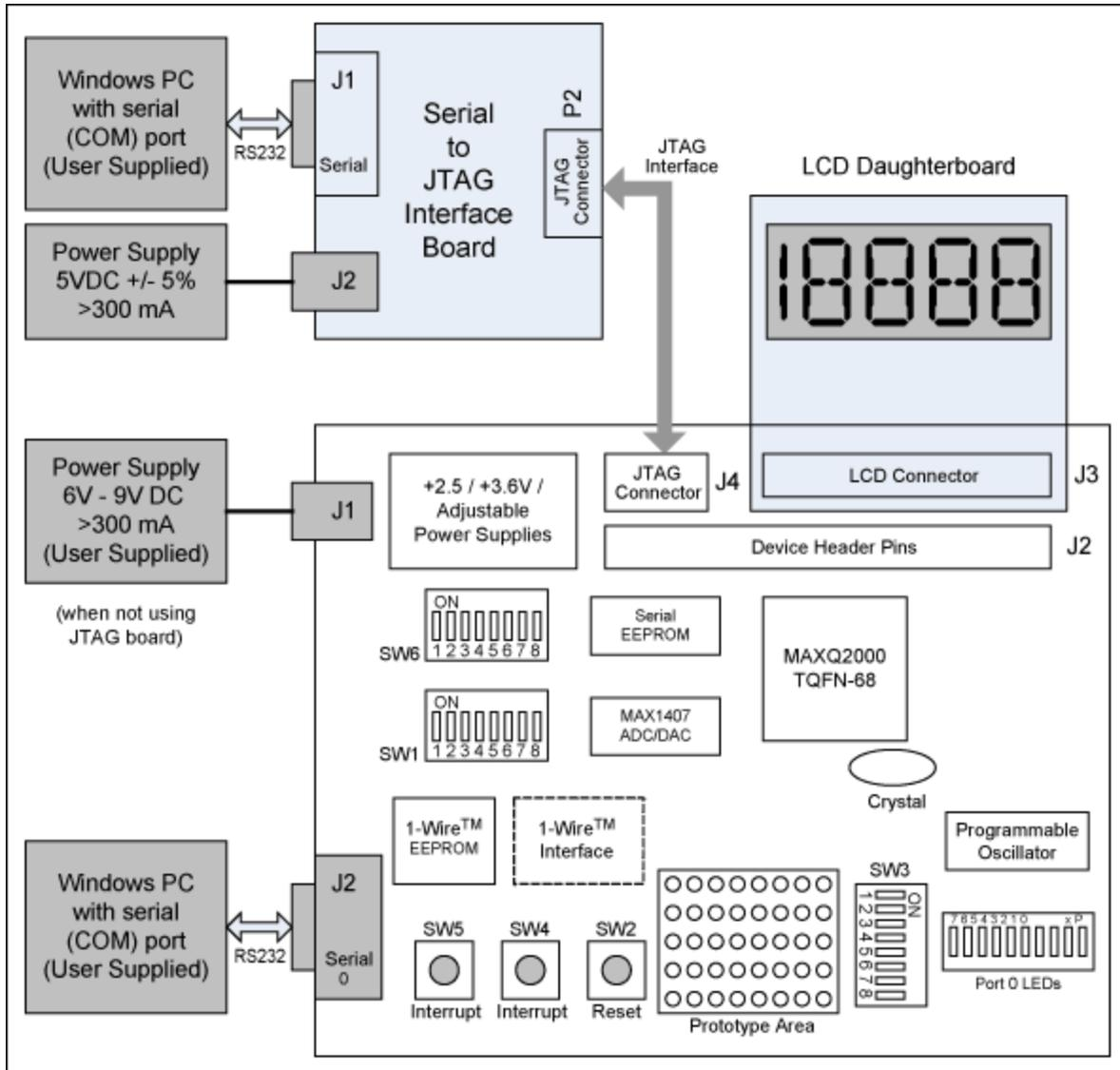
Figure 6. Block diagram for the MAXQ2000 EV kit.
