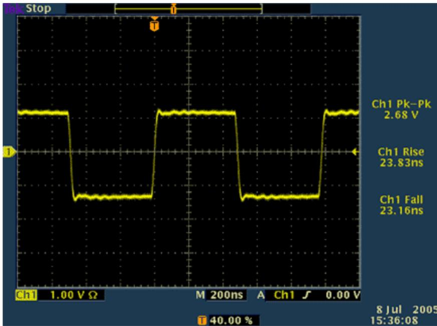
Figure 6. CMI pulse transmitted into 110Ω termination load.
