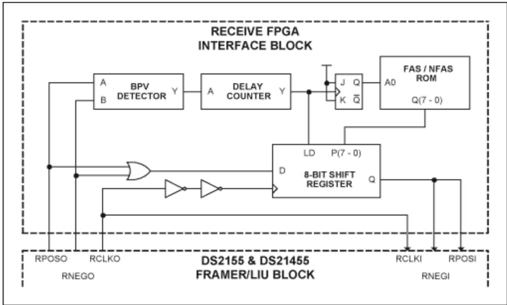
Figure 7. Diagram of a receive synchronization circuit.
