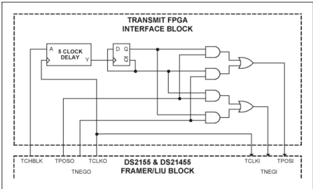
Figure 8. Diagram of a transmit bipolar violation generator.
