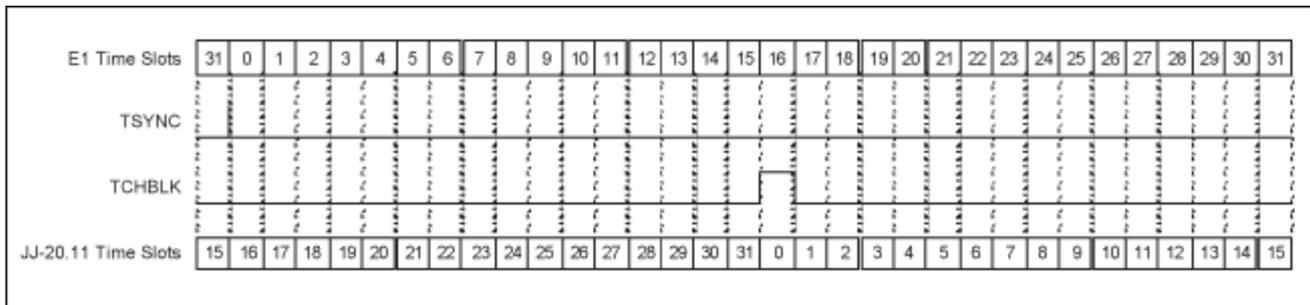
Figure 3. Transmit-side backplane timing.
