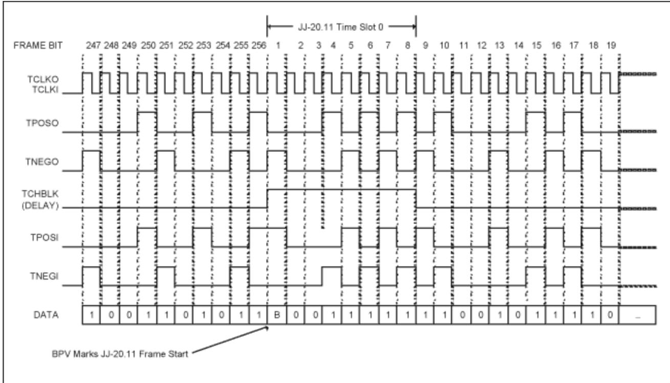
Figure 4. Transmit-side framer to LIU timing.
