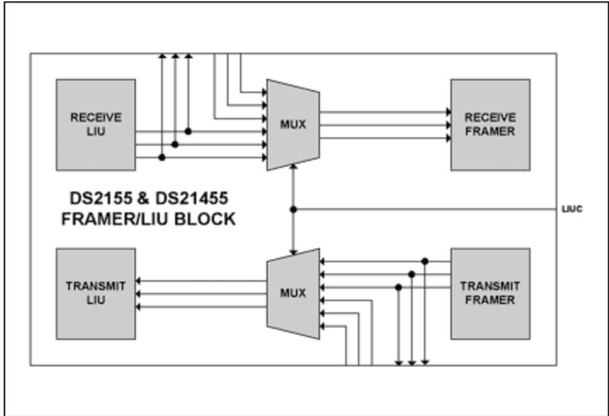
Figure 1. Simplified block diagram of DS2155 transceiver.
