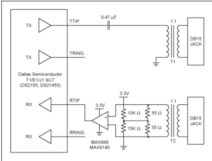
Figure 5. Illustration of a network interface circuit.
