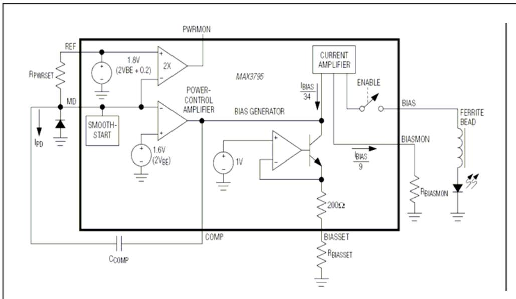
Figure 2: MAX3795 Monitor Block Diagram
