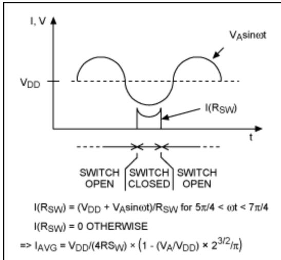
Figure 4. Switching-mode amplifier waveform.
