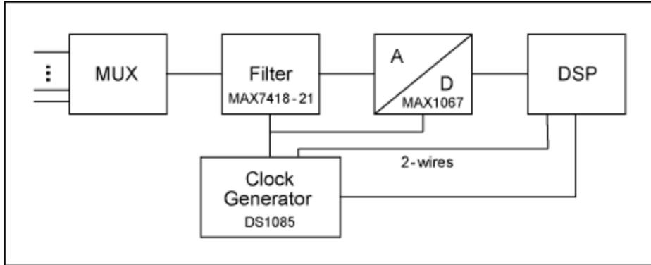
Figure 7. Schematic diagram of the realized data-acquisition system.
