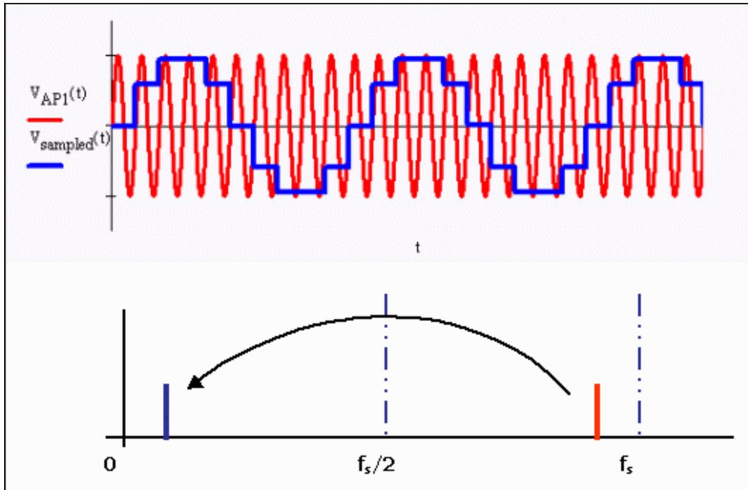
Figure 2. Aliasing in the frequency domain. A undersampled signal is mirrored at  $f_s/2$ .
