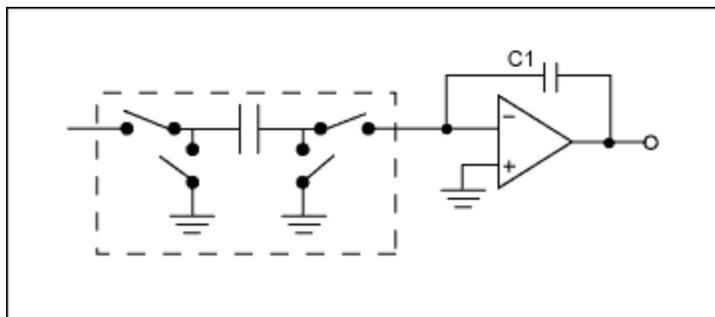
Figure 5. A simple filter realized using switched-capacitor techniques.
