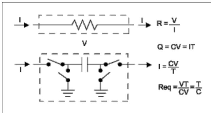
Figure 4. Switched capacitor schematic diagram.
