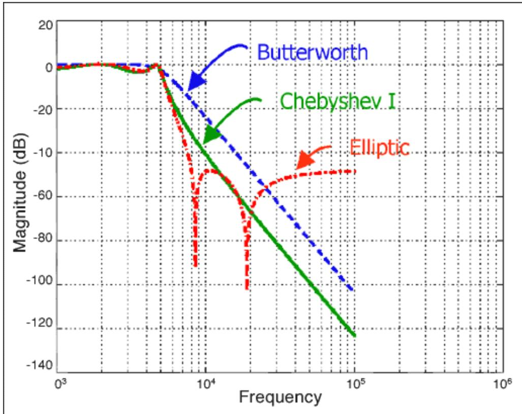
Figure 3. Comparison of different filter approximations.
