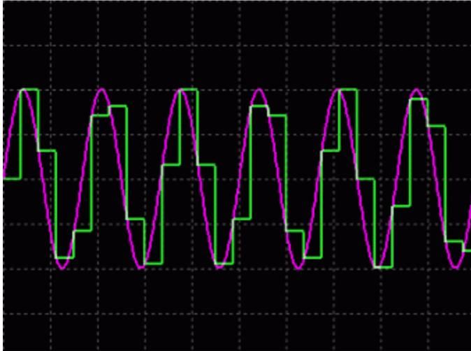
*Figure 6. Amplitude distortion caused by undersampling.*
