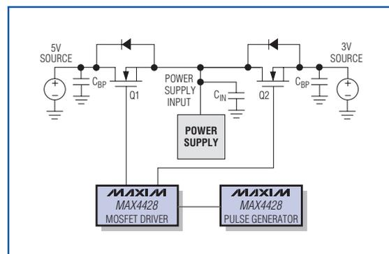
Figure 1. Two n-channel MOSFETs are shown switching between two DC sources, thus generating fast line transients.
