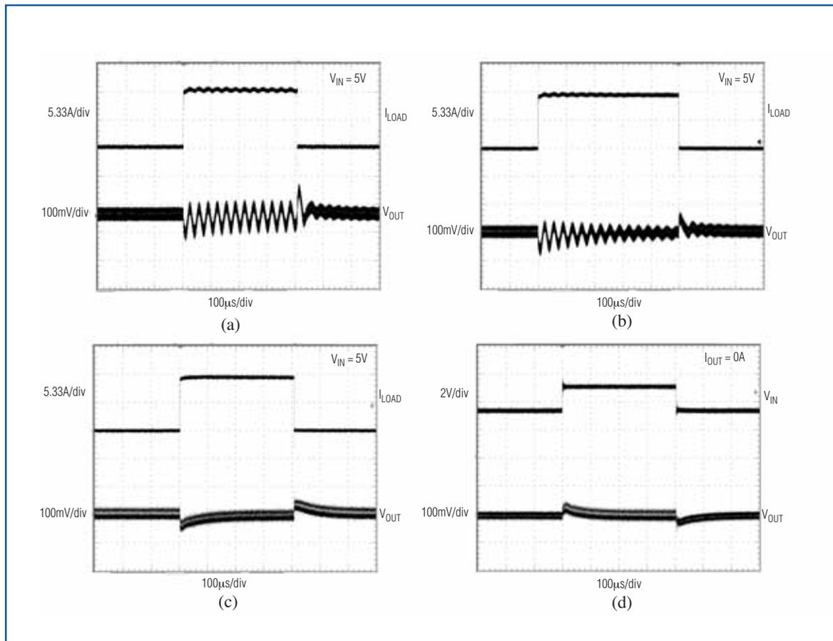
Figure 7. EV kit transient responses are shown for: a load step with 2° phase margin (a); a load step with 11° phase margin (b); a load step with 90° phase margin (c); and a line step with 90° phase margin (d).
