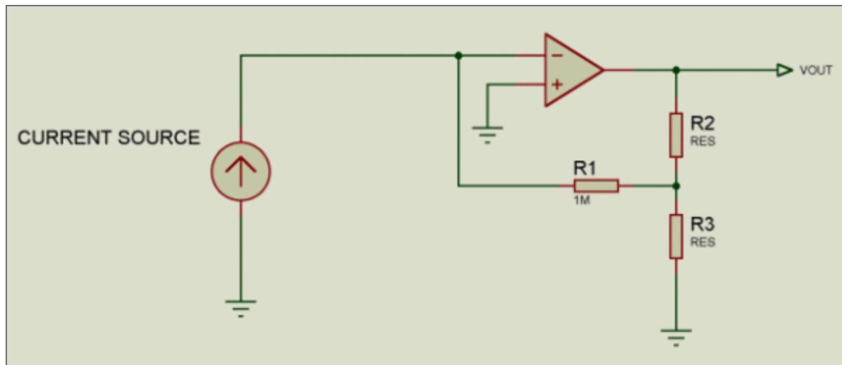
*Figure 2. Additional voltage gain in this circuit (vs. that of Figure 1) provides effective transimpedances greater than  $200\text{M}\Omega$ .*
