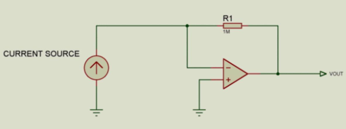
*Figure 1. For resistor values less than  $20\text{M}\Omega$ , this simple transimpedance amplifier is acceptable for use with some current sources.*
