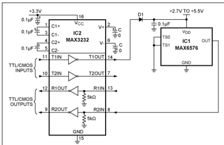
Figure 1. RS-232 powered temperature sensor.
