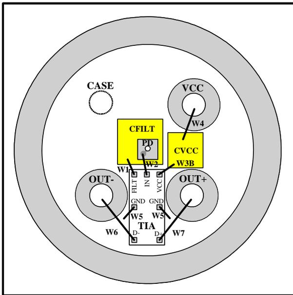
Figure 3: Top View of an improved ROSA Assembly
