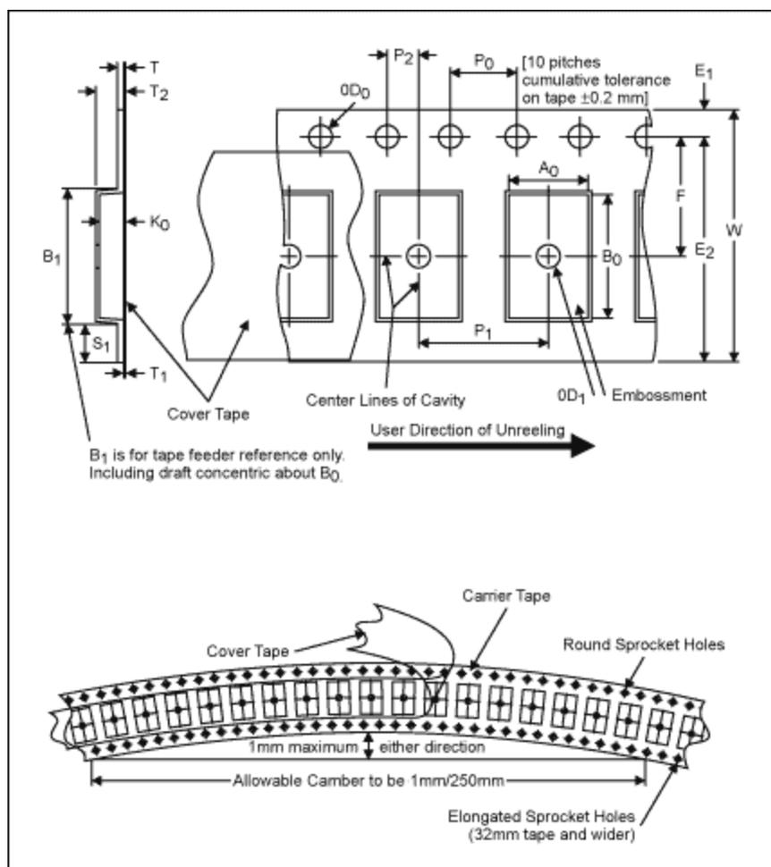
Figure 3. Typical WLP carrier tape construction.
