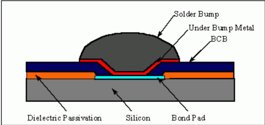
Figure 2. Cross-section diagram of generic WLP construction.
