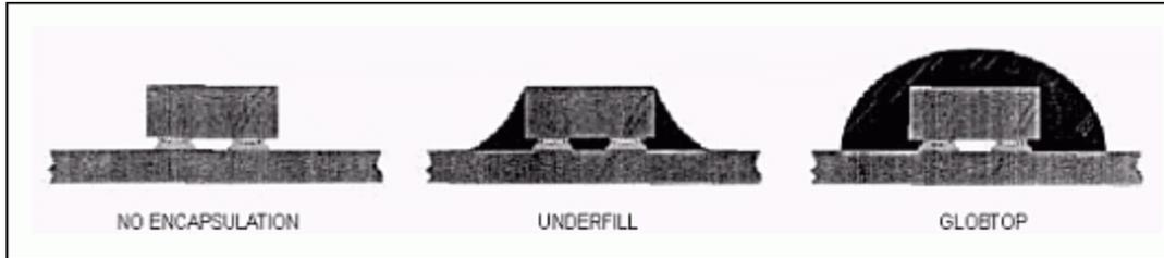
Figure 8. Epoxy encapsulation options.
