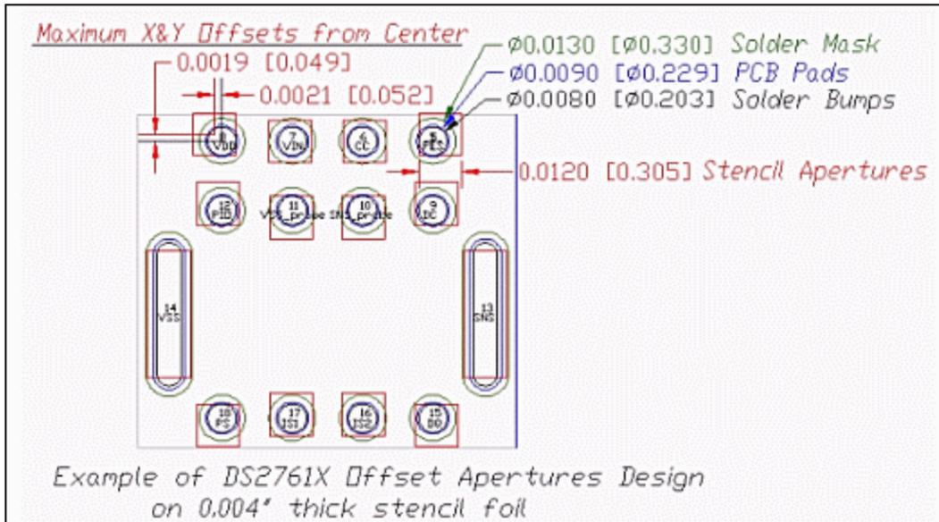
Figure 5. Example of DS2761X Flip Chip offset apertures Solder Stencil design.
