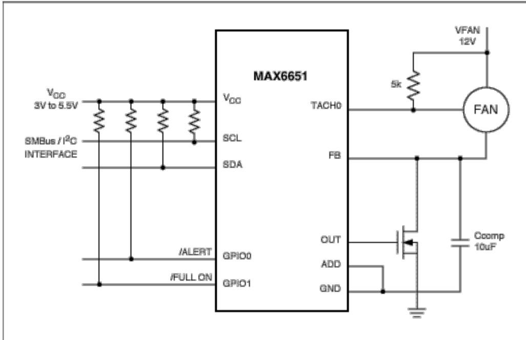
Figure 1. Normal 12V operating circuit for the MAX6651.
