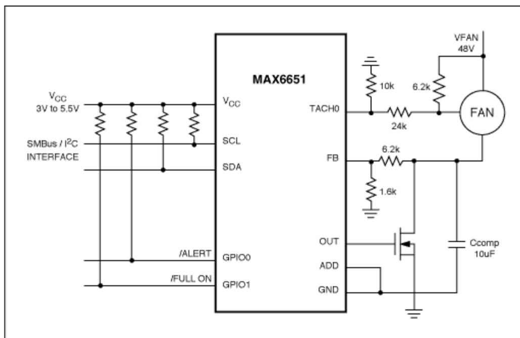
Figure 3. Driving a 48V fan with the MAX6651.
