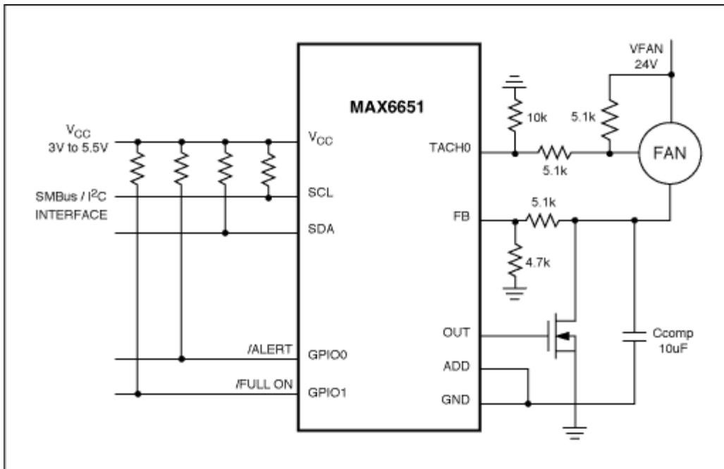
Figure 2. Driving a 24V fan with the MAX6651.
